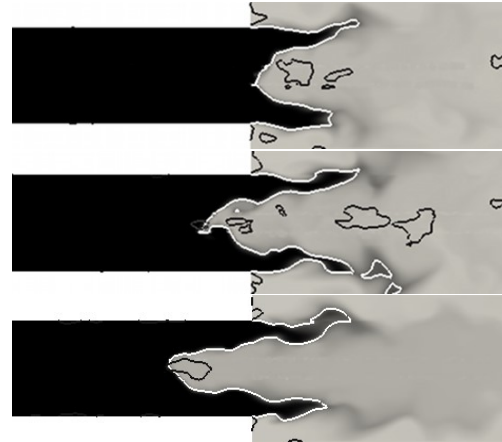
Figure 8. Reaction progress during flame flashback with BK2. Recirculation zone marked by white isoline.
