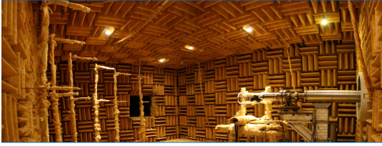
Figure 1. Anechoic chamber showing far-field microphone array (left), near-field pressure ring and PIV instrumentation (center), and axisymmetric jet (right).
