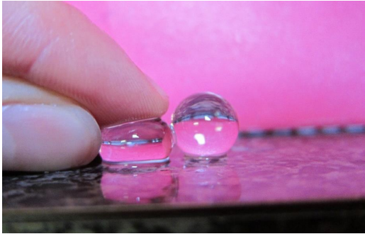
Figure 2. Super absorbent hydrogel beads upon complete saturation. Here an uncompressed bead relative to a compressed bead is shown, demonstrating the deformability of the hydrogel beads.
