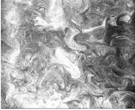
Figure 3. Example of snapshot of visualized image of horizontal plane in the logarithmic layer; flow direction is upward.
