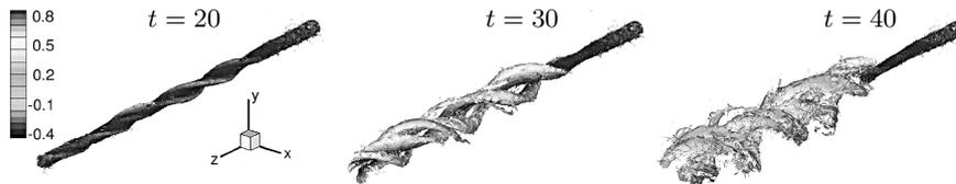
*Figure 6.* Three-dimensional temporal development of an isolated Batchelor vortex illustrating axial deceleration and formation of a stagnation point. Visualised using iso-surfaces of  $\lambda_2 = -0.4$ , shaded by axial velocity.
