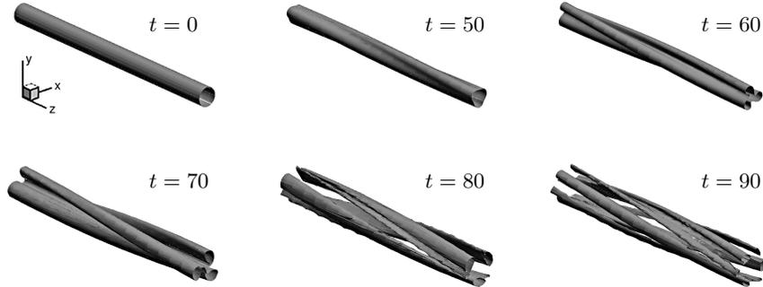
*Figure 5.* Non-linear development of an isolated Batchelor vortex assuming a periodic representation in the axial  $z$ -direction and a Fourier approximation consisting of the first 16 modes. Visualised using iso-surfaces of  $\lambda_2 = -0.2$ .
