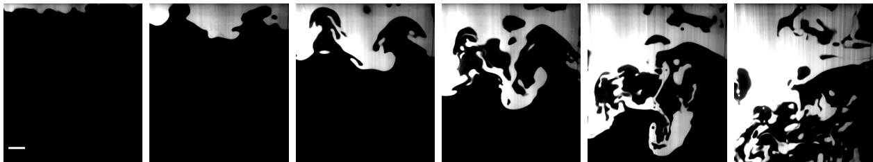
Figure 1. Snapshots of a laser induced fluorescence RT turbulence experiment (time interval between the images: 0.1 s, scale bar: 14 mm). The experiment is conducted using hexane as light fluid and a mixture of water and glycerol (37% in weight) as heavy fluid.
