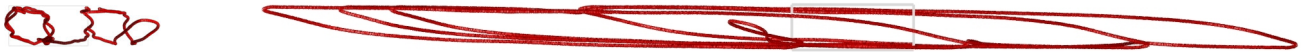
Figure 1. Trajectory of a spherical particle (diameter D/h = 0.16 , density ratio \rho_p/\rho_f = 10 ) suspended in the “gentle” Couette periodic orbit of [4] at Re = 250 and zero gravity. The temporal interval corresponds to approximately 500 bulk time units. The view is into the streamwise direction (left) and into the span (right); the grey-colored boxes indicate the domain size, while the trajectory is unwrapped in the periodic directions.
