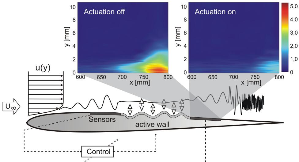
Figure 2. Fluctuations within the boundary layer with actuation off (left contour plot) and actuation on (right contour plot)
