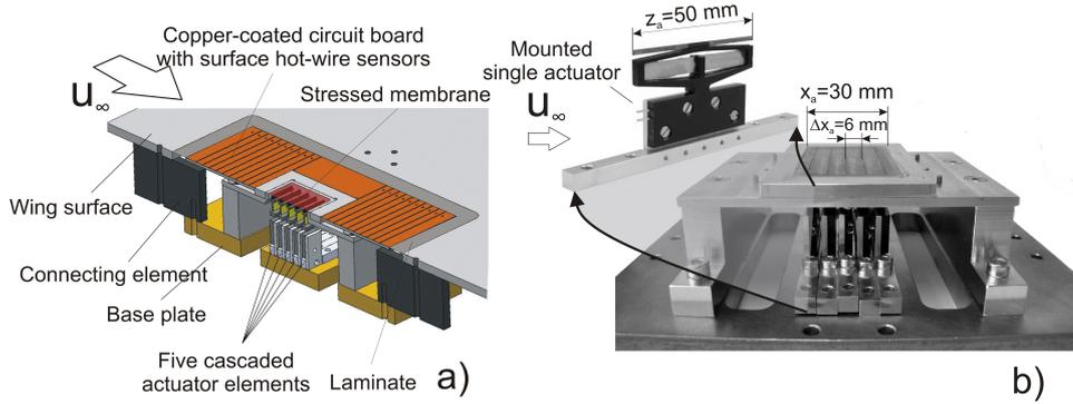
Figure 1. Active wall, driven by five streamwise actuator elements, (a) Sketch of sensor actuator set-up (b) Photo of this installation
