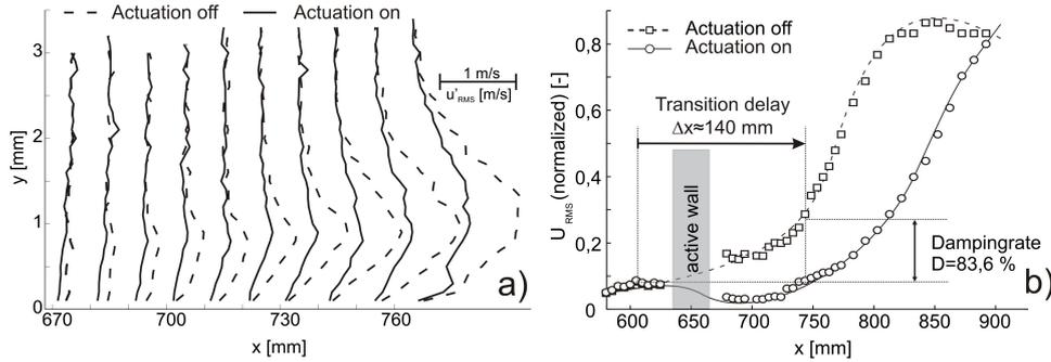
Figure 3. Boundary layer downstream of the actuated wall (a) boundary layer profile of velocity fluctuations, (b) Amplification of the TS-Wave and transition delay
