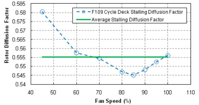
**Figure 8. F109 Overall Map Stall Line Rotor Diffusion Factor**
