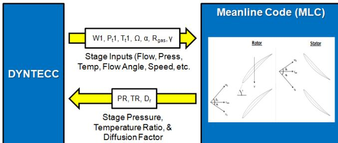
**Figure 5. Operation of DYNTECC Using a MLC to Provide Local Stage Pressure and Temperature Characteristic Information at Each Time Step**
