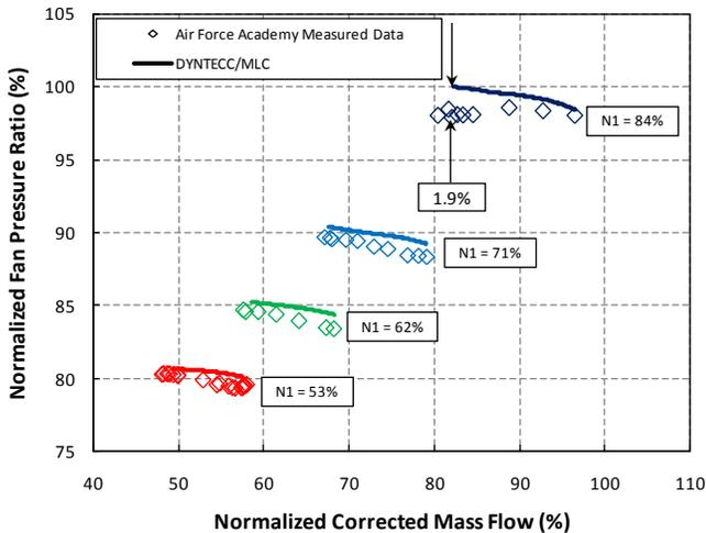
Figure 10. DYNTECC/MLC Predicted and USAFA Measured Fan Map Comparison (No Swirl)
