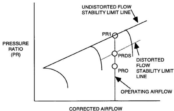
Figure 13. Loss in Stability Pressure Ratio ( $\Delta PRS$ ) [4]
