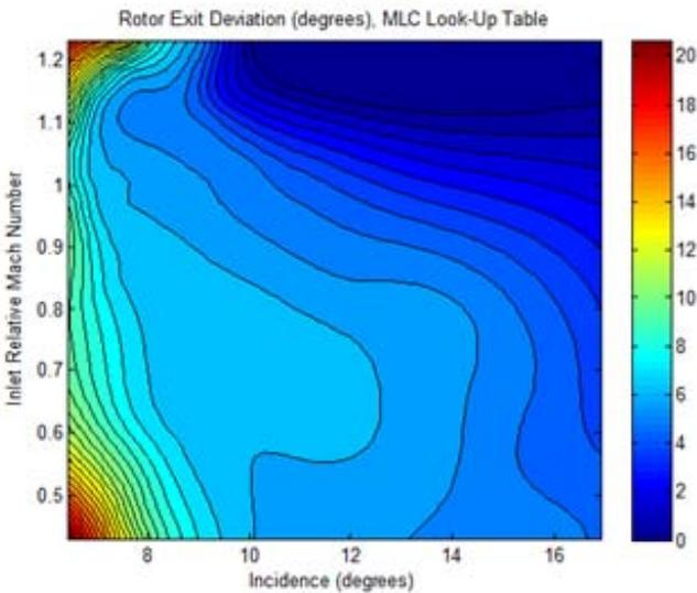
**Figure 7. Relative Rotor Deviation**
