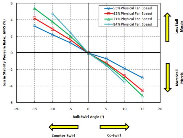
**Figure 16. Loss in Stability Pressure Ratio ( $\Delta$ PRS) as a Function of Bulk Swirl Angle**
