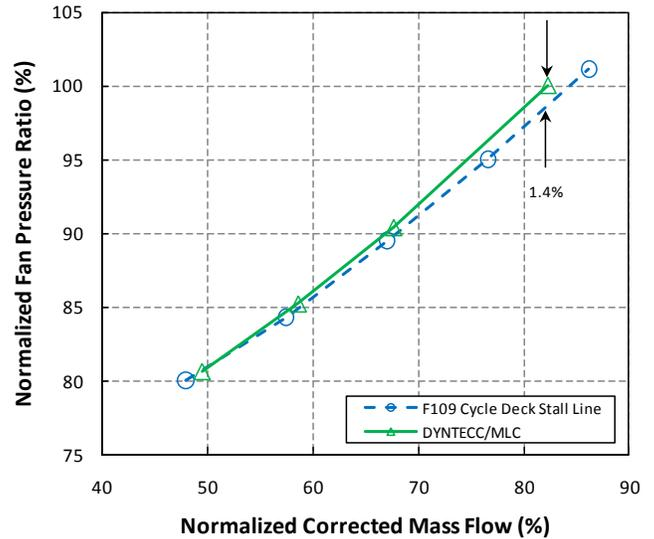
Figure 11. DYNTECC/MLC Predicted and F109 Cycle Deck Specified Fan Stall Line (No Swirl)
