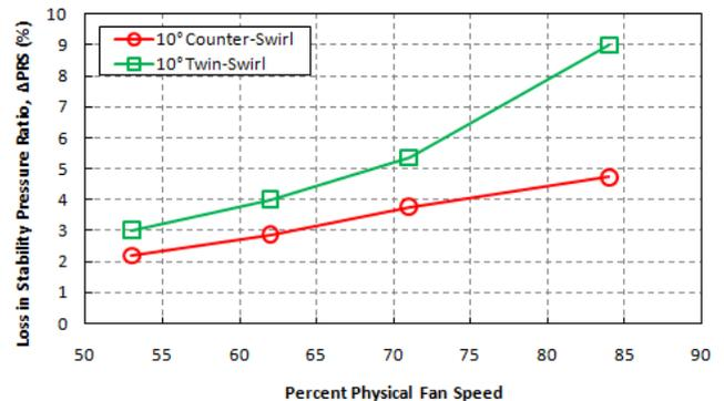
**Figure 18. Loss in Stability Pressure Ratio ( $\Delta$ PRS) as a Function of Percent Referred Fan for 10° Counter-Swirl and 10° Twin-Swirl**
