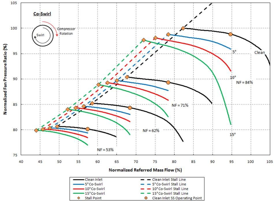
Figure 14. DYNTECC/1-D MLC Prediction of the Effect of Co-Swirl on F109 Fan Performance and Operability
