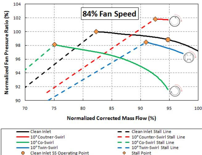
**Figure 17. DYNTECC/1-D MLC Prediction of the Effect of 10° Co-Swirl, 10° Counter-Swirl and 10° Twin-Swirl on F109 Fan Performance and Operability at 84% Fan Speed**
