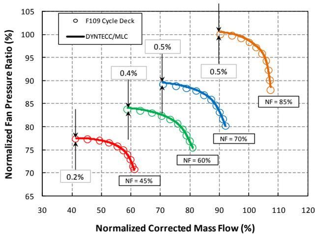
Figure 9. DYNTECC/MLC Predicted and F109 Cycle Deck Specified Fan Map Comparison (No Swirl)
