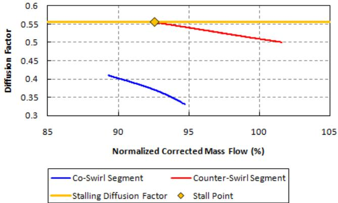
Figure 19. Twin Swirl Segment Diffusion Factor at Constant Fan Speed
