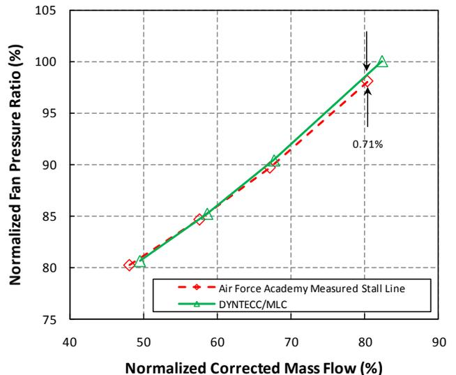
Figure 12. DYNTECC/MLC Predicted and USAFA Measured Fan Stall Line (No Swirl)
