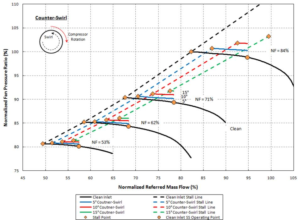
Figure 15. DYNTECC/1-D MLC Prediction of the Effect of Counter-Swirl on F109 Fan Performance and Operability
