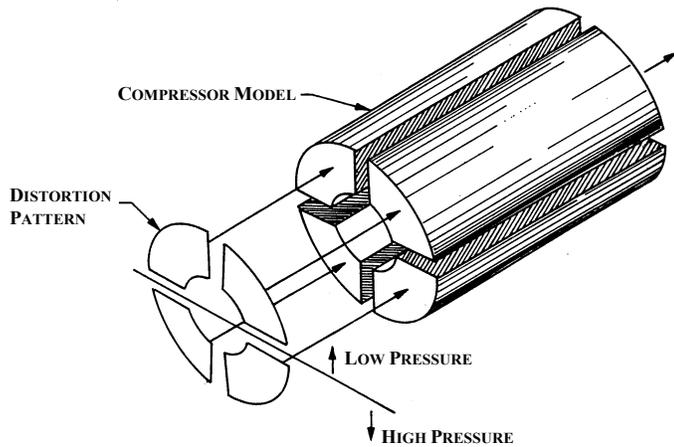
**Figure 3. Parallel Compressor Theory Concept [16]**
