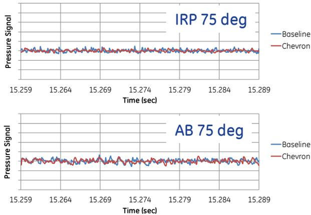
**Figure 21 Pressure Signal Time Series from Engine Test at 134 ft., for IRP and AB Engine Conditions at 75 deg.**
