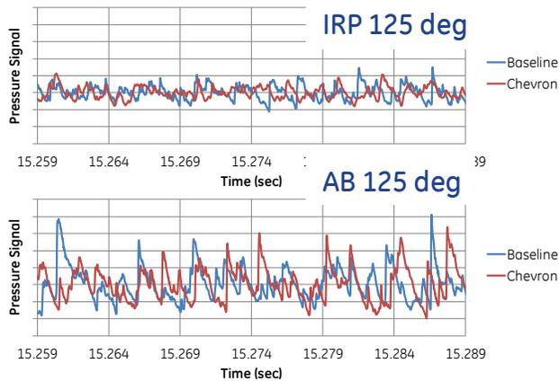
**Figure 22 Pressure Signal Time Series from Engine Test at 134 ft., for IRP and AB Engine Conditions at 125 deg.**
