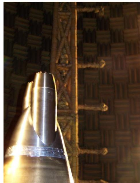
**Figure 15 Photo of Twin Nozzle and Farfield Microphone Array in the Background.**
