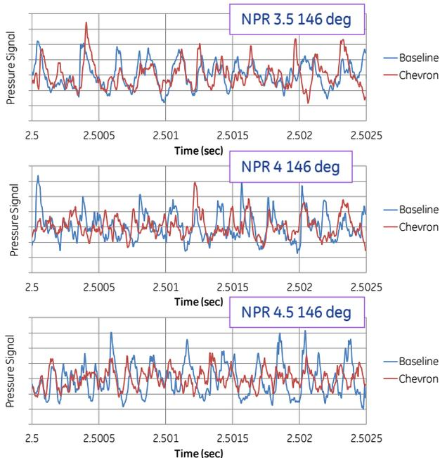
**Figure 28 Pressure Signals from Scale Model Test at 16.5 in for Three Nozzle Pressure Ratios at 146 deg.**
