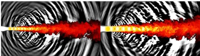
Figure 10 LES of an over-expanded jet;  $Tr=1.74$ ,  $M_{jet}=1.35$ .
