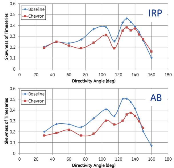
**Figure 23 Skewness of pressure signal from Engine Test at 134 ft., for IRP and AB Engine Conditions.**
