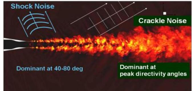
**Figure 8 Shock and Crackle noise components of supersonic jets.**
