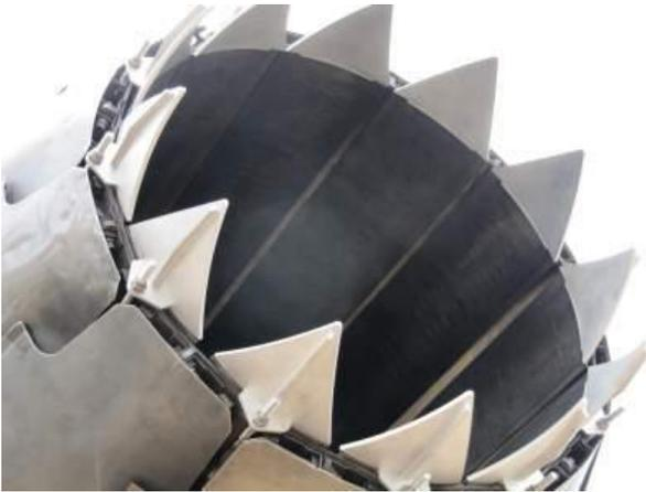
**Figure 13 Close-up Photo of Engine Exhaust Nozzle and Chevrons.**
