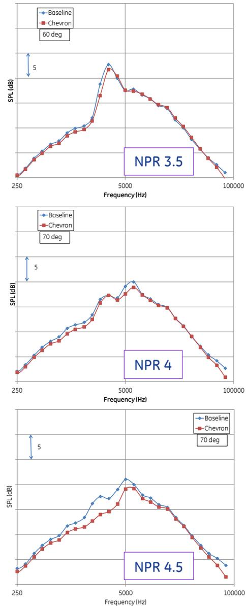
**Figure 25 SPL Spectra from Scale Model Test at 22 ft. for Three Nozzle Pressure Ratios.**
