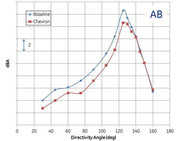
**Figure 18 dBA Directivity from Engine Test at 134 ft., for IRP and AB Engine Conditions.**
