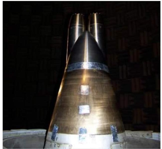
**Figure 14 Photo of Twin Nozzle Simulation of Installed F414 Configuration.**
