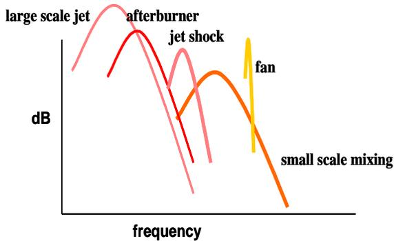
**Figure 6 Typical tactical aircraft noise sources relative amplitudes.**
