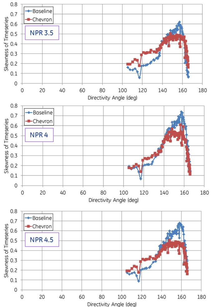
**Figure 29 Skewness of pressure signal from Scale Model Test at 16.5 in for Three Nozzle Pressure Ratios.**
