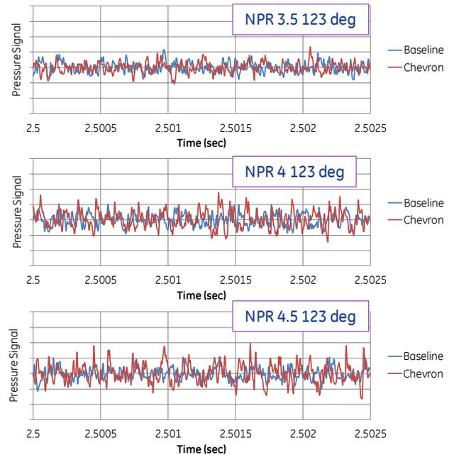
**Figure 27 Pressure Signals from Scale Model Test at 16.5 in for Three Nozzle Pressure Ratios at 123 deg.**
