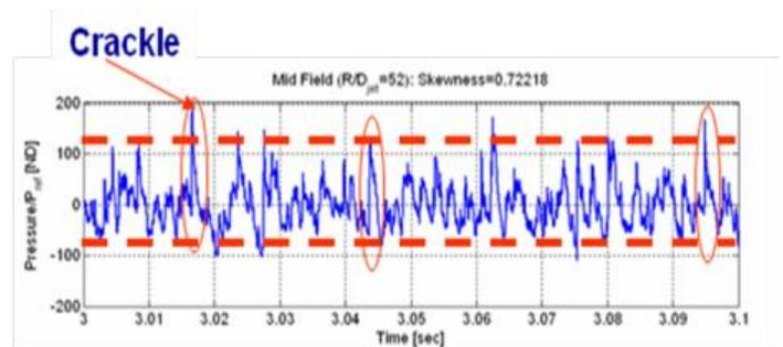
**Figure 9 Crackle waveform of a typical tactical aircraft engine [6].**
