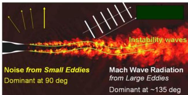
**Figure 7 The two components of supersonic jet mixing noise.**
