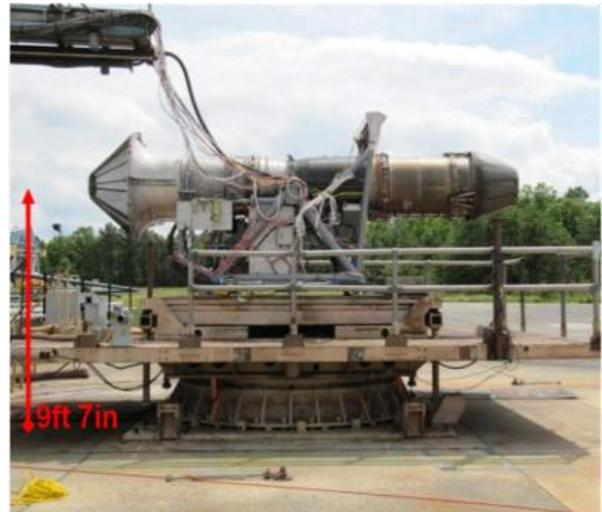
Figure 11 Photo of F404 Engine on Test Stand During Test.
