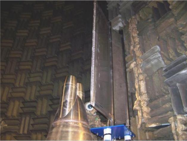
**Figure 16 Photo of Twin Nozzle and Nearfield Array.**
