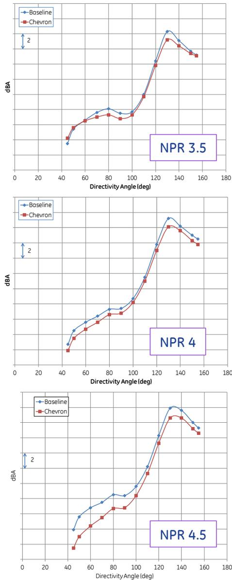
**Figure 24 dBA Directivity from Scale Model Test at 22 ft., for Three Nozzle Pressure Ratios.**
