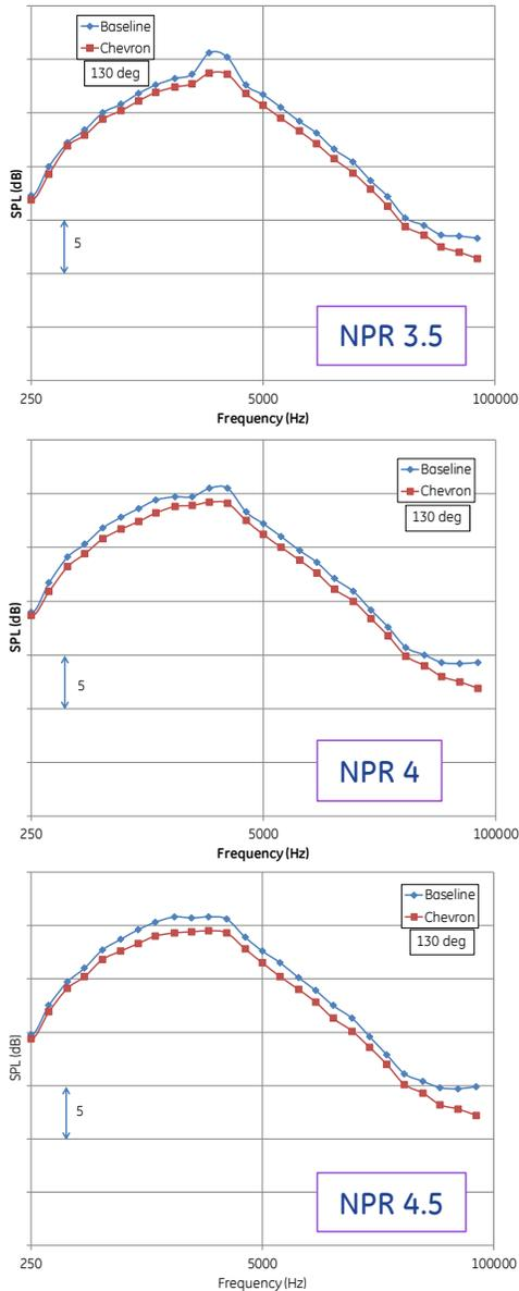
**Figure 26 SPL Spectra from Scale Model Test at 22 ft. for Three Nozzle Pressure Ratios at 130 deg.**
