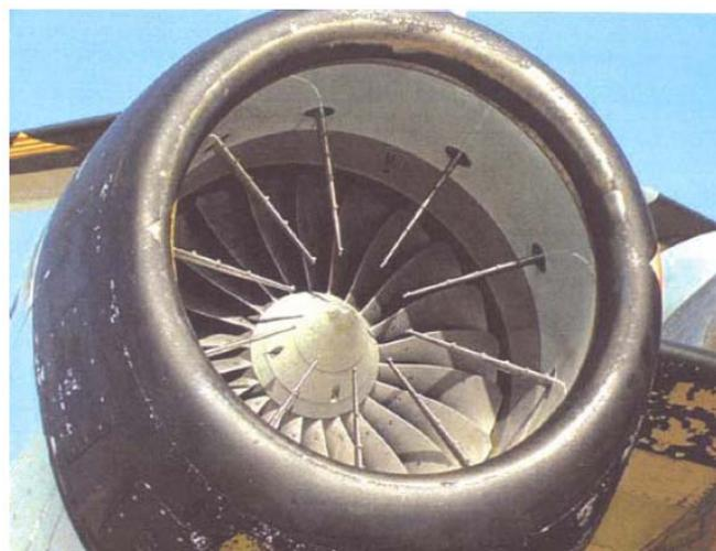
**Figure 19 : HTF7000 Inlet Distortion Rake Schematic and 10 Rake, 6 Immersion Installation in a HTF7000 Inlet.**
