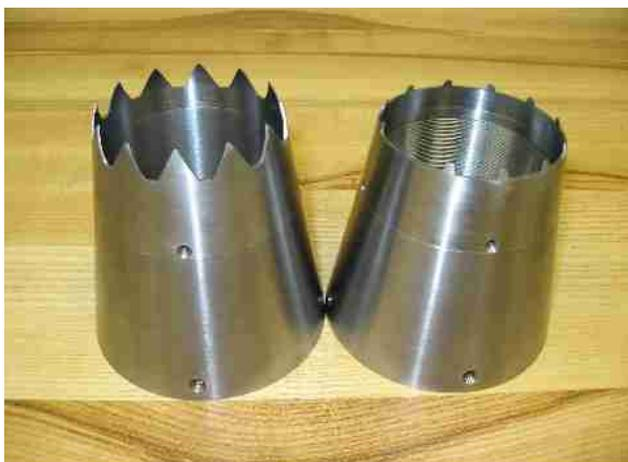
**Figure 13. Nozzles for Noise / Performance Tradeoff**
