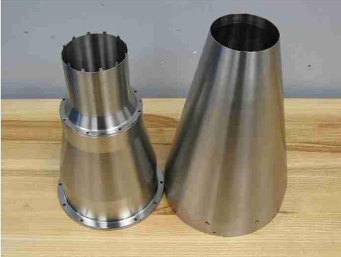
**Figure 1. Convergent-Divergent Exhaust Nozzle**
