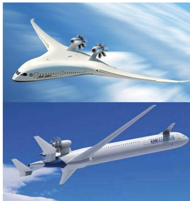
Figure 2. Notional Open Rotor Airplane Concepts [14][15].
