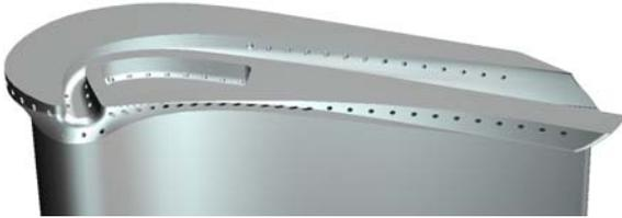
**Fig. 2 Geometry of Cooled Winglet Tip**
