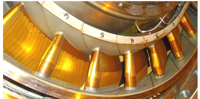
Figure 12: Completed and Installed Vane Ring Photo taken after a yearlong series of blowdown testing
