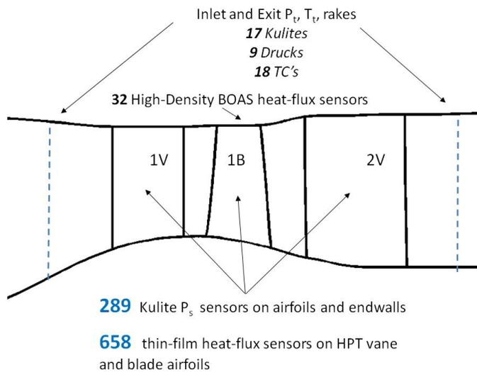
Figure 3: Instrumentation Requirements for the HIT Research Turbine
