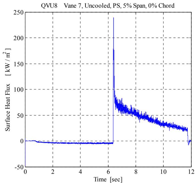
Figure 23: Surface Heat Flux Trace Calculated from Double-Sided Thin Film Signals in Figure 22
