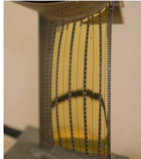
Figure 9: Trailing Edge Looking Upstream of a Cooled Vane with Sensors Near the ID Endwall
