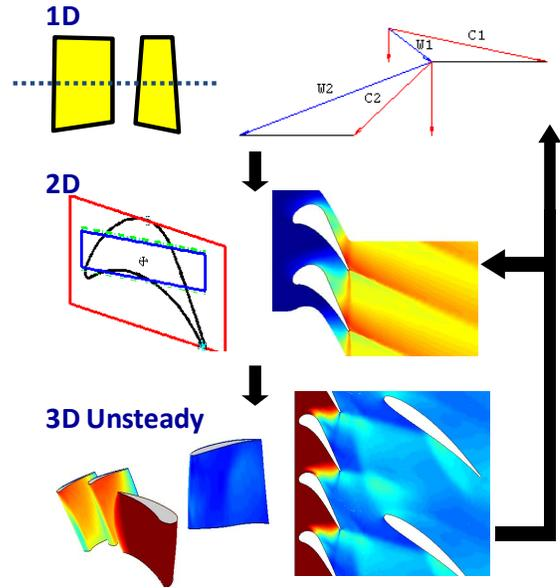
Figure 2: A Typical Iterative Design Loop for Turbine Airfoils.
