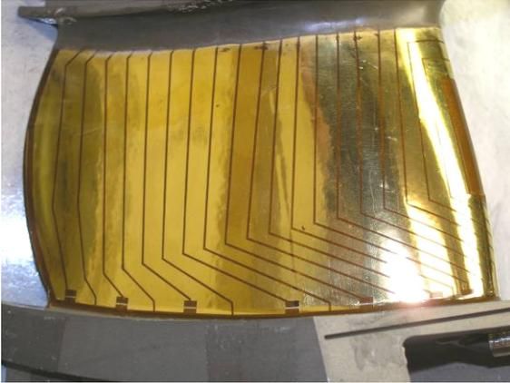
Figure 10: Double-Sided Vane Sensors Near OD Endwall
