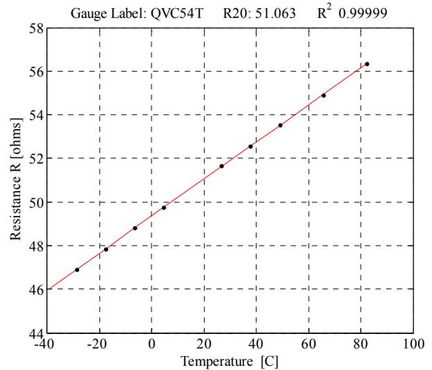
Figure 5: Thermal Calibration Points for a Single Thin Film Sensor
