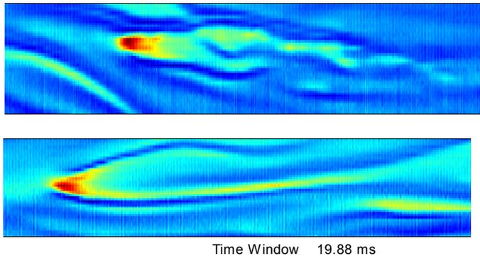
Figure 17: Example Time-Resolved Heat Flux Data from a High Density Heat Flux Imaging Array on a Leading Edge Subjected to Freestream Turbulence (Anthony et. al. [31])
