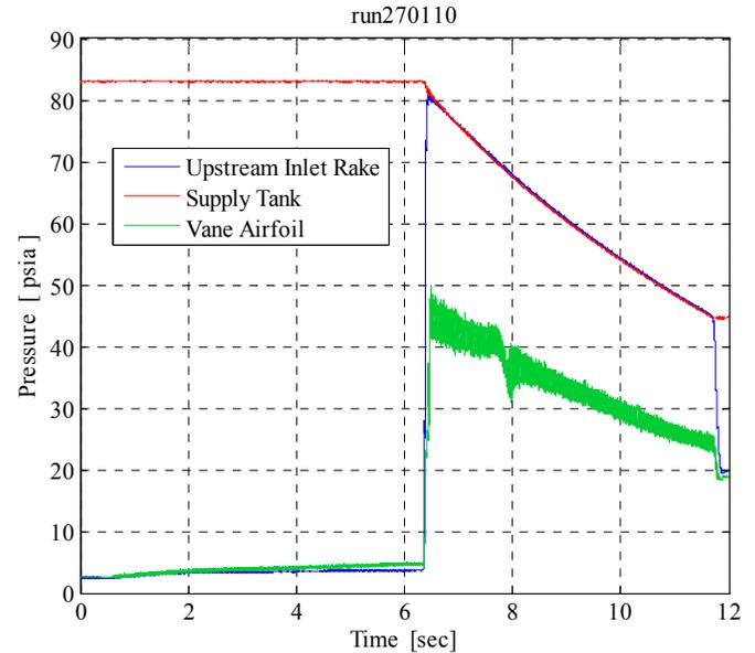
Figure 21: Pressures During TRF Blowdown with an Initial Precool Period
