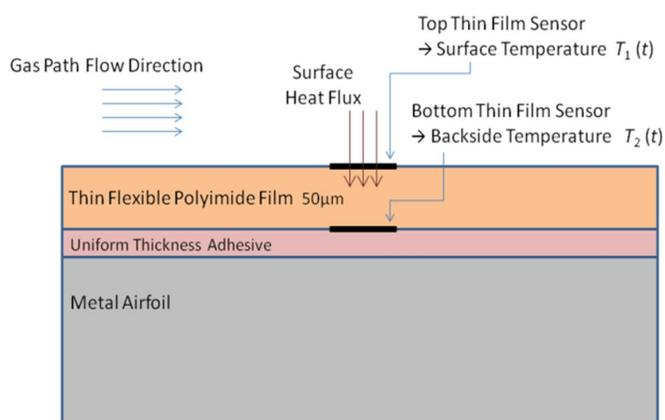
Figure 7: Double-Sided Thin Film Heat Flux Sensor Diagram
