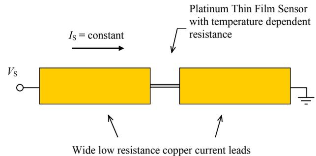
Figure 4: Schematic of a conventional thin film heat flux sensor
