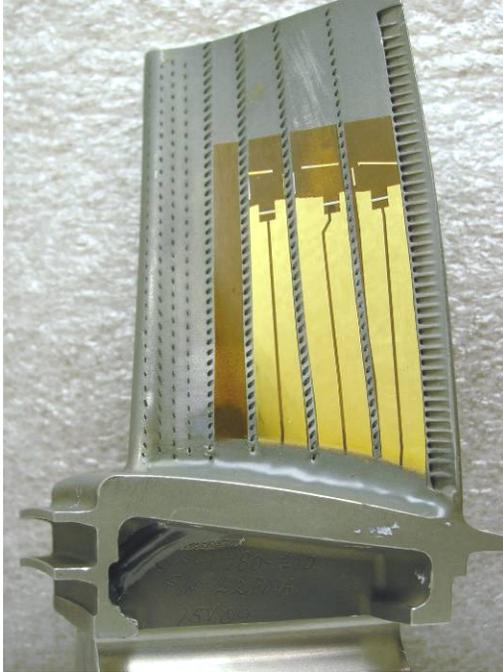
Figure 13: Cooled Pressure Side Rotor Blade with Double-Sided Films
