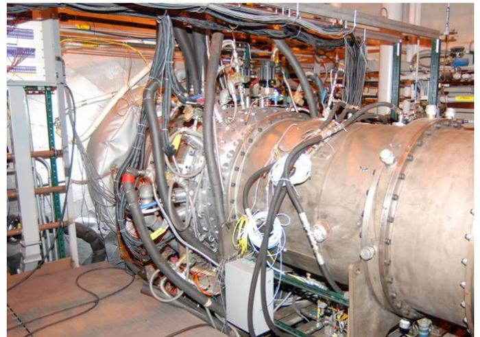
Figure 19: Test Section of the AFRL Turbine Research Facility with the Cooled Research Turbine Vane Installed for Testing
