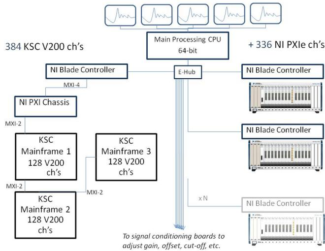
Figure 20: Updated Data Acquisition Expansion Scalable to Higher Channel Count
