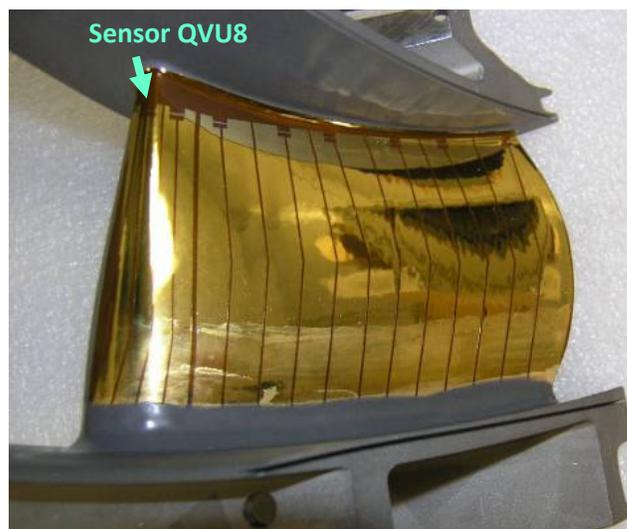
Figure 8: Double-Sided Vane Sensors Near the ID Endwall
