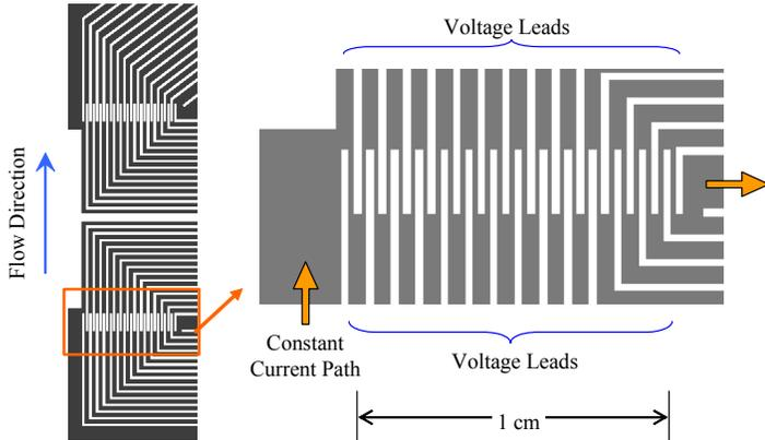
Figure 16: Schematic of a High Density Heat Flux Imaging Array
