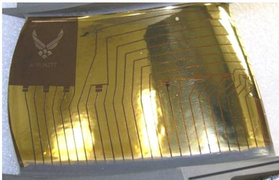
Figure 11: Double-Sided Vane Sensors Along 50% Span
