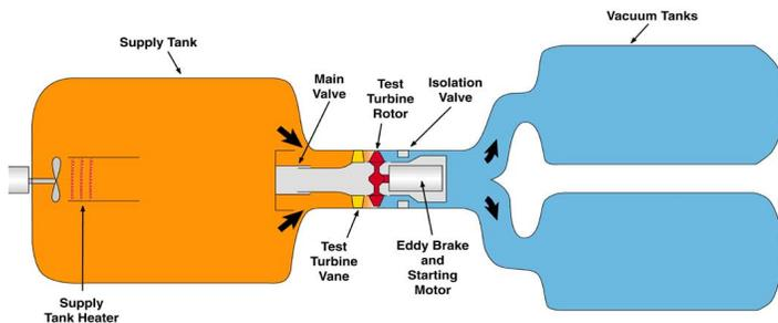
Figure 18: Diagram of the Turbine Research Facility at WPAFB
