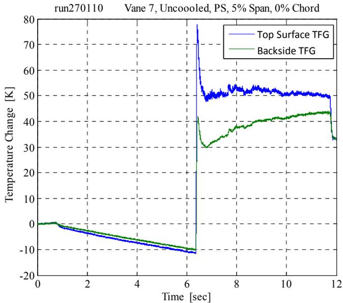
Figure 22: Double-Sided Thin Film Temperature Traces From a Vane Test Run with Pre-Cooling and Main Valve Open Just After 6 Seconds
