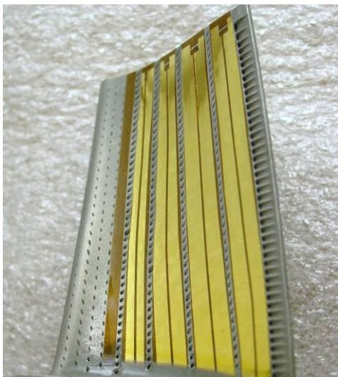
Figure 14: Sensors Near the Tip of a Fully Cooled Rotor Blade
