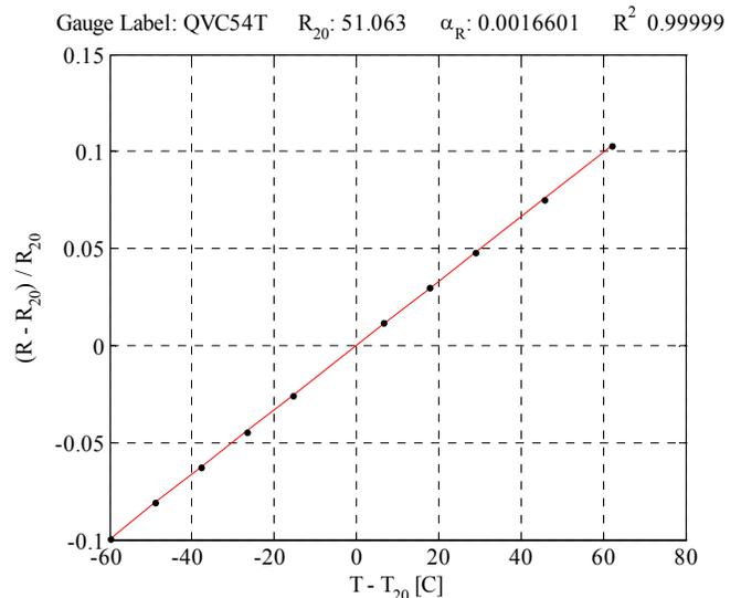
Figure 6: Thermal Coefficient of Resistance  $\alpha_R$  determined for each individual sensor
