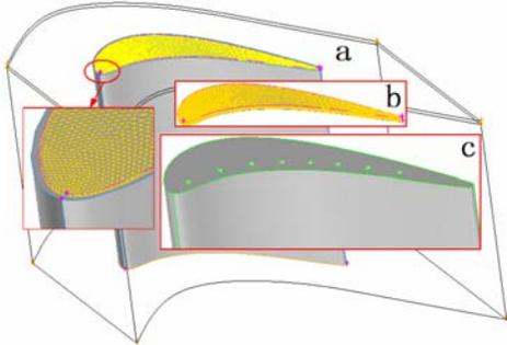
Fig. 12 Structure of (a) squealer tip blade, (b) cavity, (c) flat tip blade
