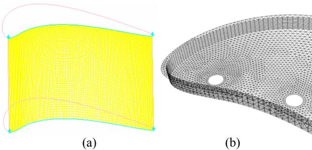
Fig. 4 Grid feature of (a) pressure surface, (b) tip groove surface
