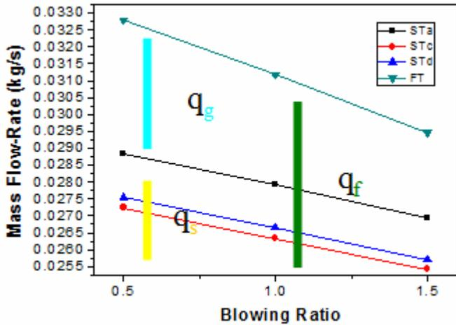
Fig. 13 The mass flow rates of the leakage flow in different blade tip models (STa, STc, STd and FT) with different blowing ratios (0.5, 1 and 1.5)
