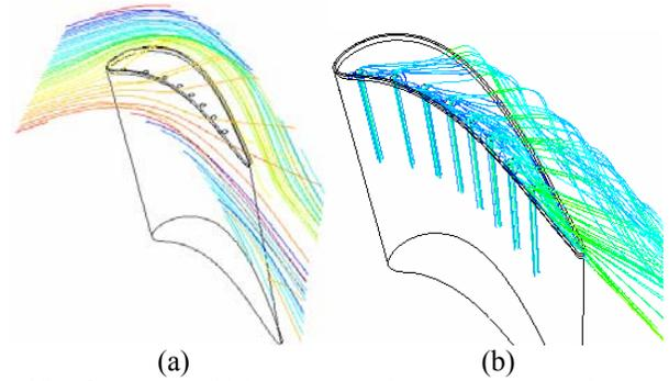
Fig. 10 Path lines of (a) tip leakage flow on squealer tip and (b) coolant
