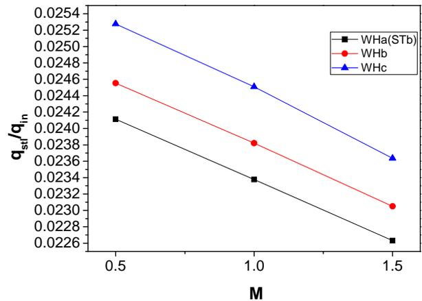
Fig. 19 The mass flow ratios of the leakage flow in different rim widths (STb, WHb and WHc) and different blowing ratios (0.5, 1 and 1.5) [19]
