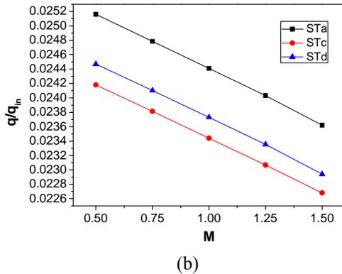
Fig. 16 The mass flow ratios of the leakage flow of (a) flat tip and squealer tip, and (b) squealer tip with different blowing ratios (0.5, 0.75, 1, 1.25 and 1.5)
