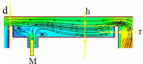
Fig. 15 Influence factors of leakage flow
