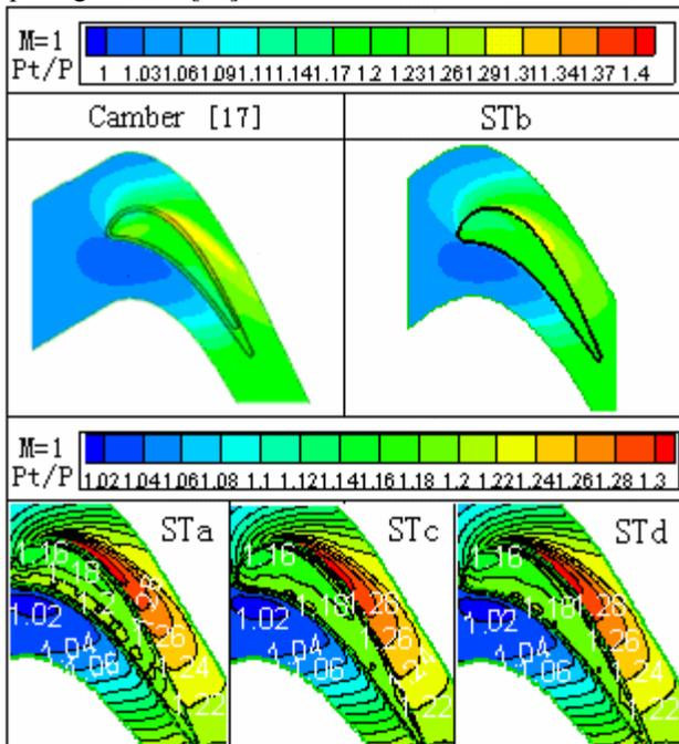
Fig. 9 Comparisons of Pt/P value on shroud with Yang et al. [17], different configurations(STa, STb, STc and STd), M=1
