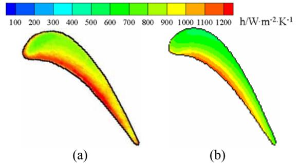
Fig. 8 Comparisons of  $h$  value on flat tip ( $M=1.0$ ) (a) experimental result [14], without film holes, (b) present simulation, without film holes
