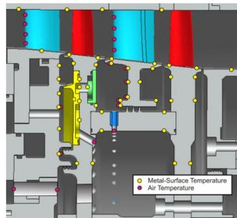
**Figure 6: Temperature Measurement Locations**
