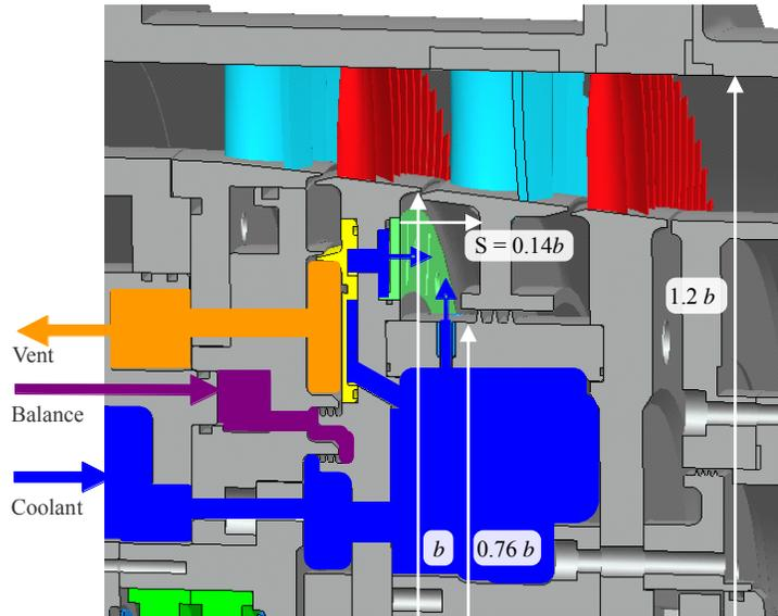
**Figure 3: Internal Air System Schematic**
