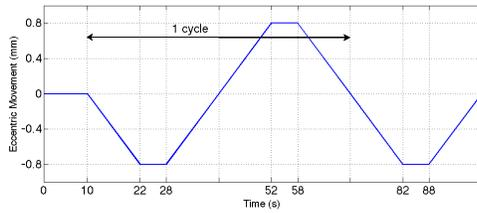
Figure 4. Displacement cycles used to characterise seal
