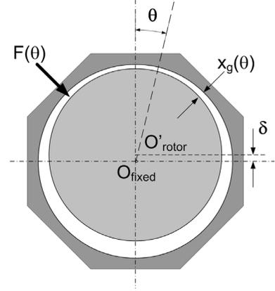
Figure 10. Eccentric rotor schematic.
