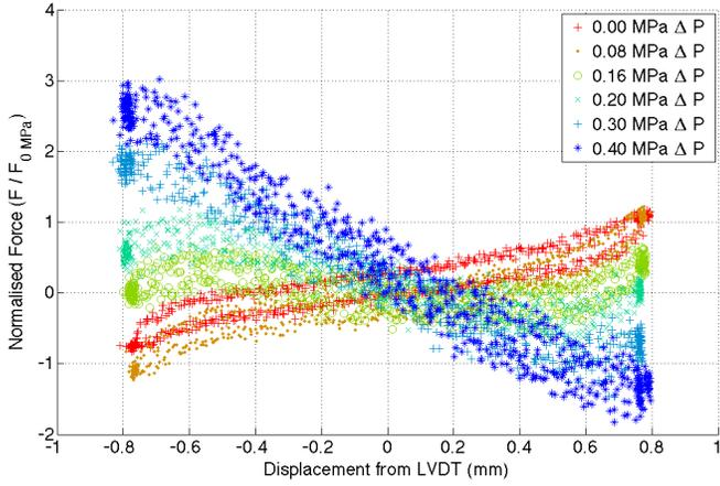
Figure 6. Composition of force-displacement cycles at different pressures (intermediate pressures have been omitted for clarity).
