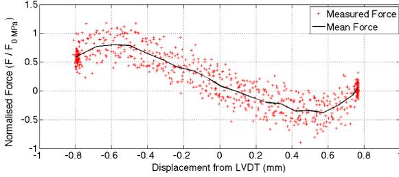
Figure 7. Force versus displacement plot at 0.2MPa (test 6).
