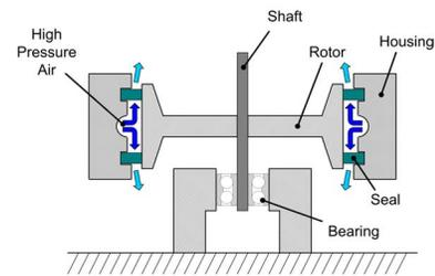
Figure 2. Facility cross section
