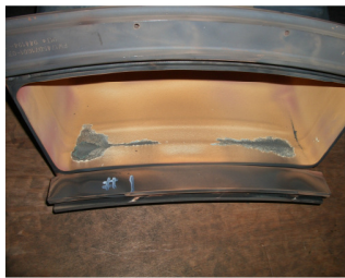
(a) Failure of Lower panel (b) Crack on the corner region
