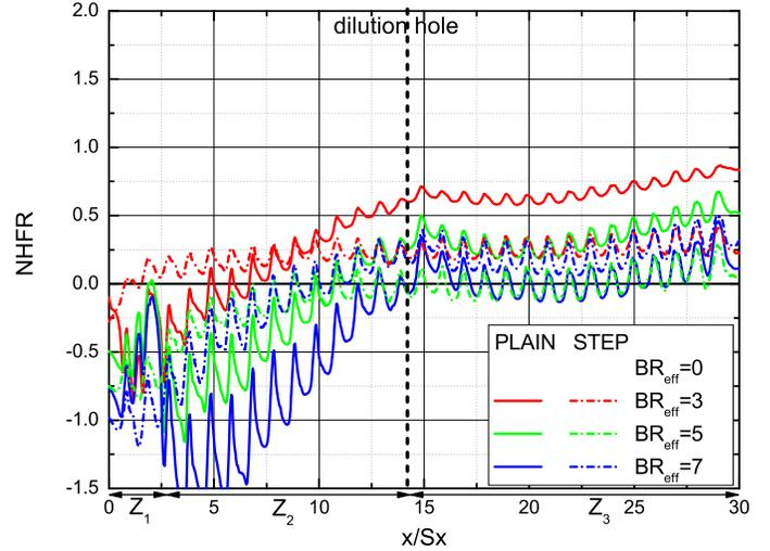
Figure 9. SPANWISE AVERAGED NHFR WITH ONLY EFFUSION COOLANT
