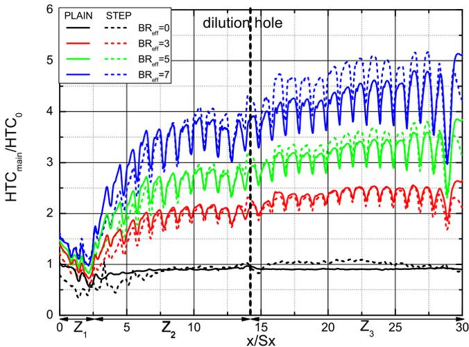
Figure 5. SPANWISE AVERAGED HTC WITH SLOT AND EFFUSION COOLANT
