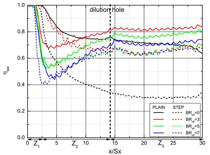
Figure 8. SPANWISE AVERAGED  $\eta_{aw}$  WITH SLOT AND EFFUSION COOLANT
