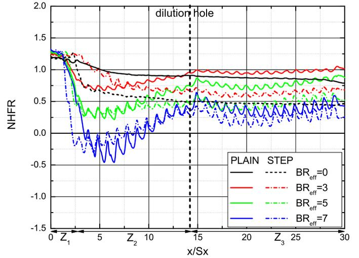
Figure 10. SPANWISE AVERAGED NHFR WITH SLOT AND EFFUSION COOLANT
