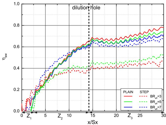
Figure 7. SPANWISE AVERAGED  $\eta_{aw}$  WITH ONLY EFFUSION COOLANT
