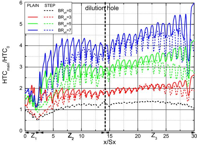
Figure 4. SPANWISE AVERAGED HTC WITH ONLY EFFUSION COOLANT
