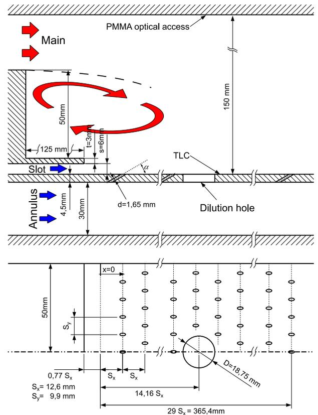
Figure 2. LINER GEOMETRY
