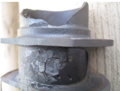
Figure No.11 Cross firing tube metals broken by quenching.
