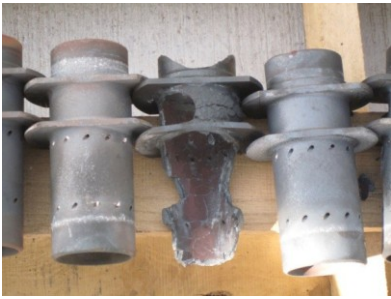
Figure No.8 Melted and broken material of cross firing tube bodies.
