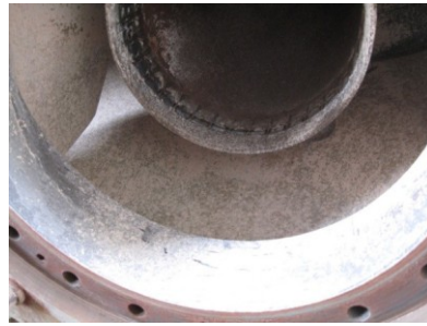
Figure No.12 White scale patterns sprayed on the transition piece.
