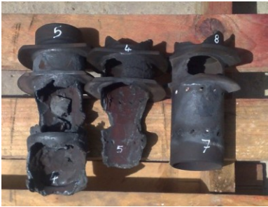
Figure No.9 Broken and melted material from cross firing tube bodies.
