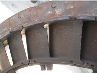
Figure No.17 Signs of broken metal and dents on first stage turbine nozzles upper half.
