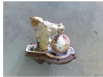
Figure No.23 Water trap valve cover and plunger covered with white solidified element (desiccant).
