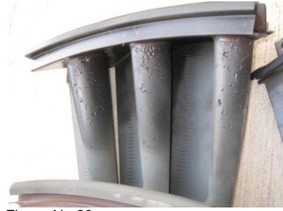
Figure No.20 Signs of dents on second stage turbine nozzles.
