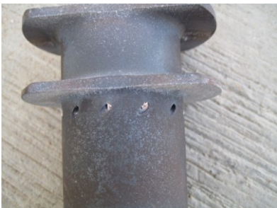
Figure No.10 Cross firing tube air cooling passes blocked with white scale.
