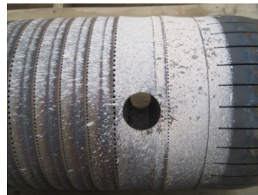
Figure No.6 White scale covering the combustion liner air passes.
