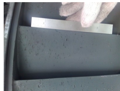
Figure No.15 Second stage turbine nozzles scaling the dents.
