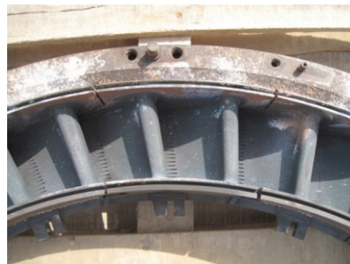
Figure No.13 White scale element and burnout on first stage turbine nozzles bottom half.
