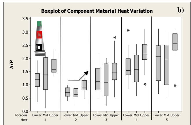
Figure 9. Component Material a) master heat variation and b) location variation.
