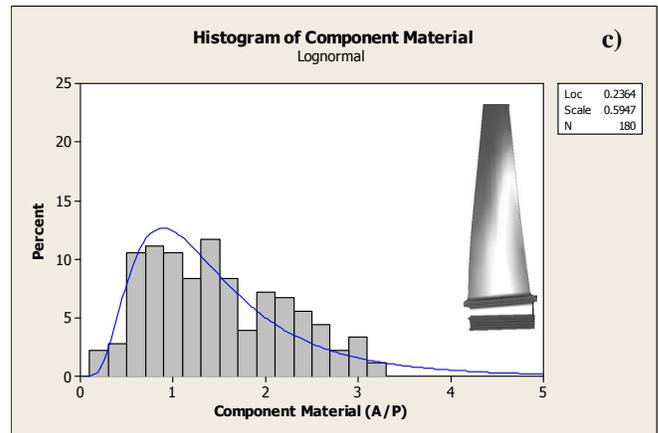
**Figure 4. Histograms of a) Engineering Design Database, b) Qualification tests, and c) Machined from component tests.**
