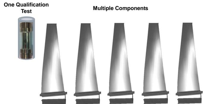
**Figure 2. A single Qualification test approves material Master Heat (batch) for use in multiple parts.**
