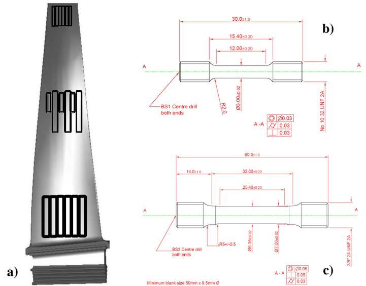
**Figure 3. Machined from component specimen location template, and specimens drawings.**
