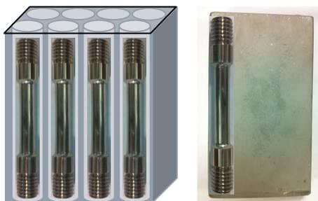
**Figure 1. Engineering Design Database generated from separately cast slab/bar material.**
