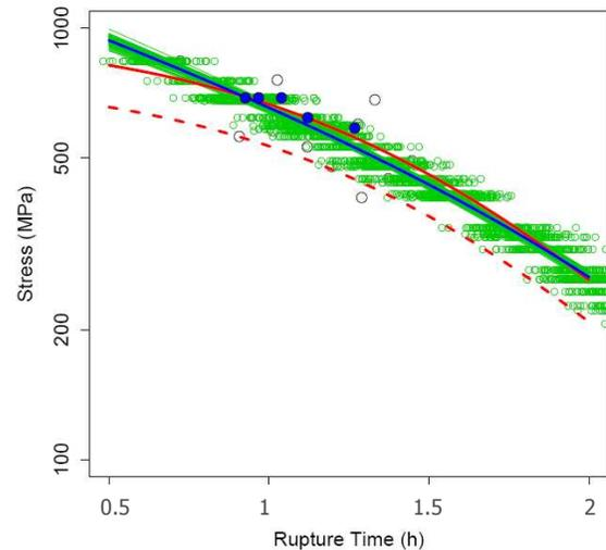
Figure 10. Uncertainty of Curve Fit of Normalized Engineering Database Material
