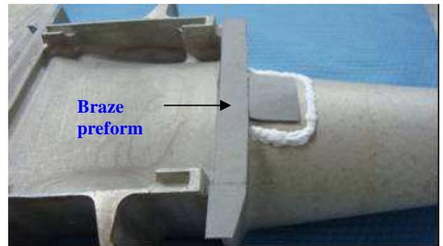
Figure 24 – Application of braze preform for suction side platform build up
