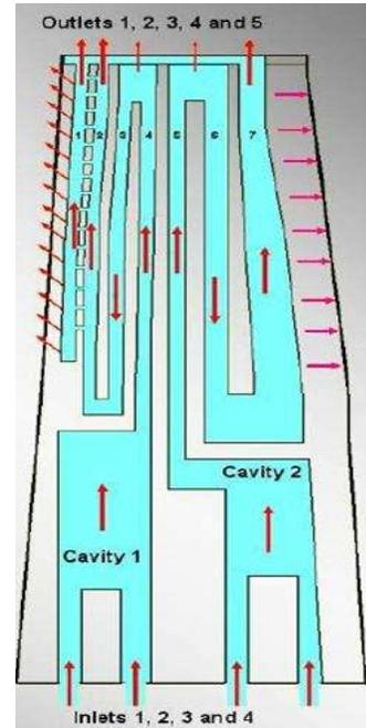
**Figure 1 – Schematic of internal serpentine passages of the Frame 7FA, stage 1 bucket (Ref. 3)**
