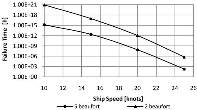
Figure 11: Turbine creep life variation – Weather conditions (mid-temperature profile and f1-hull fouling)
