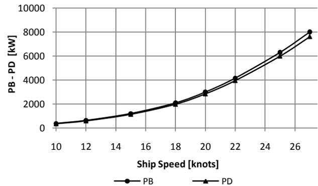
Figure 5: Brake power and delivered power variation – Ship speed (2 beaufort, mid-temperature profile and f1-hull fouling)
