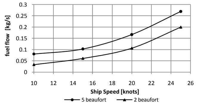
Figure 9: Fuel flow variation – Weather conditions (mid-temperature profile and f1-hull fouling)
