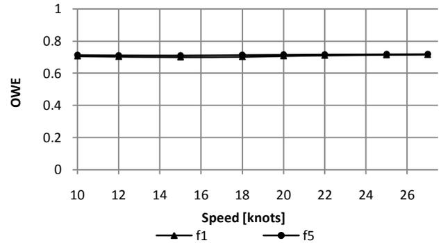
Figure 8: Open water efficiency variation – Ship speed (2 beaufort and mid-temperature profile)
