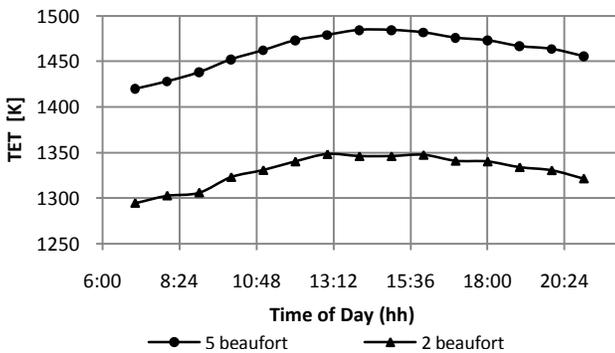
Figure 12: Turbine entry temperature variation – Weather conditions (mid-temperature profile, f1-hull fouling and 20 knots)
