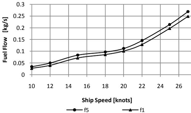
Figure 3 : Fuel flow variation – Ship speed (2 beaufort and mid-temperature profile)
