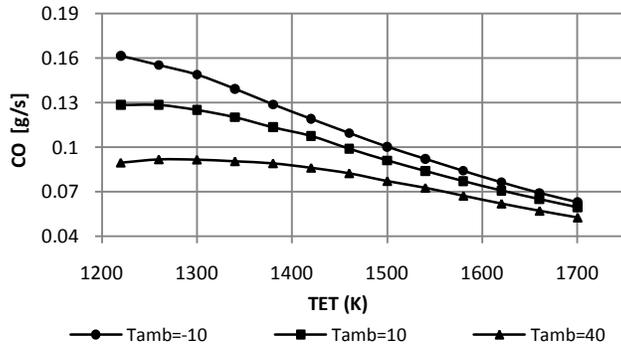
Figure 15: CO exhaust emissions variation – TET (2 beaufort and f1-hull fouling)
