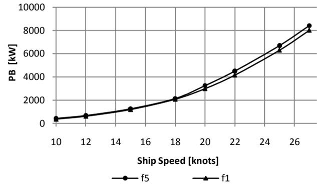
Figure 4: Brake power variation – Ship speed (2 beaufort and mid-temperature profile)
