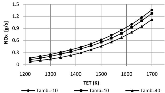
Figure 14: NO<sub>x</sub> exhaust emissions variation – TET (2 beaufort and f1-hull fouling)
