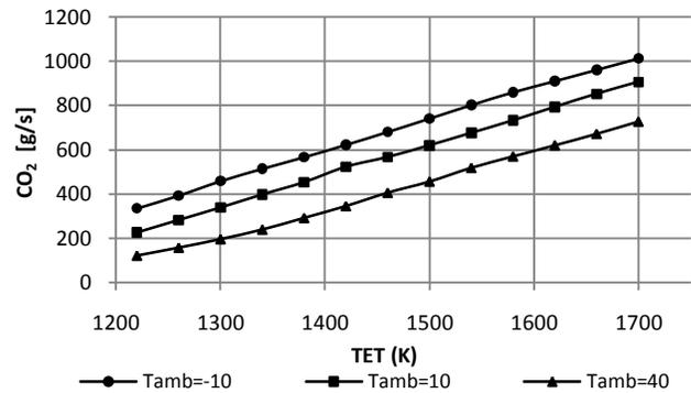
Figure 13: CO<sub>2</sub> exhaust emissions variation – TET (2 beaufort and f1-hull fouling)
