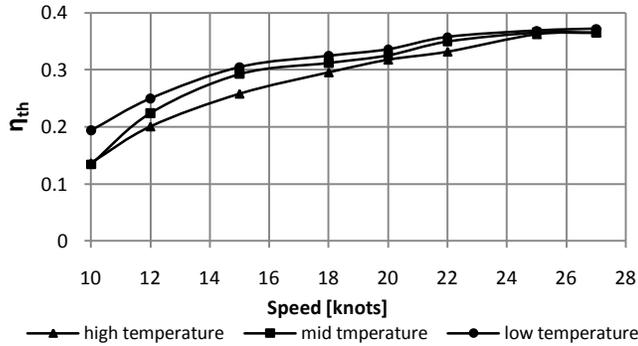
Figure 6: Thermal efficiency variation – Ship speed (2 beaufort and f1-hull fouling)
