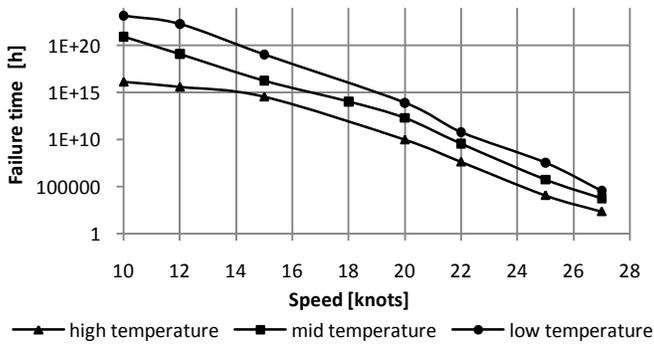
Figure 7: Turbine creep life (failure time) – Ship speed (2 beaufort and f1-hull fouling)
