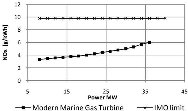
Figure 20:  $NO_x$  exhaust emissions for distillate fuel
