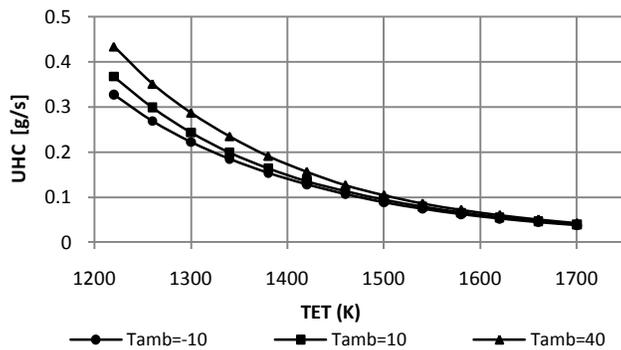
Figure 16: UHC exhaust emissions variation – TET (2 beaufort and f1-hull fouling)
