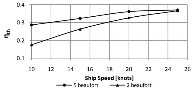
Figure 10: Thermal efficiency variation – Weather conditions (mid-temperature profile and f1-hull fouling)
