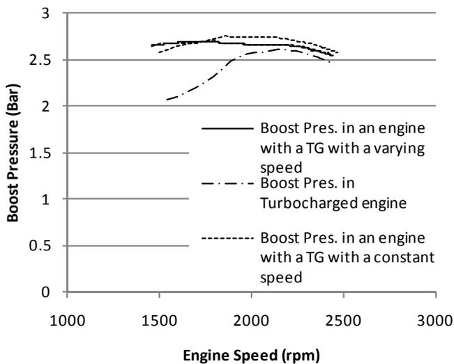
Figure 16. BOOST PRESSURE AS A FUNCTION OF ENGINE SPEED
