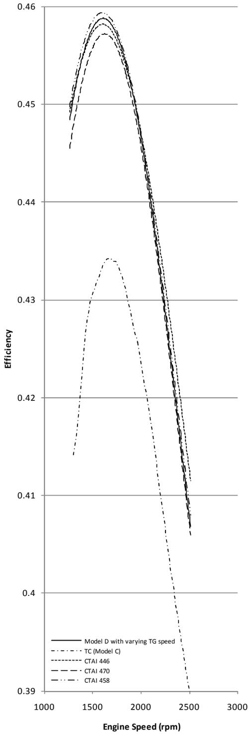
**Figure 13. HOW OVERALL EFFICIENCY IS AFFECTED BY INLET VALVE TIMING**
