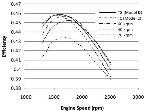
**Figure 9. OVERALL SYSTEM EFFICIENCY FOR DIFFERENT TURBOGENERATOR SPEEDS DURING ENGINE SPEED TRANSIENT**
