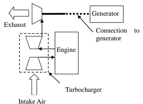
**Figure 1. Typical layout of a Turbogenerated engine**
