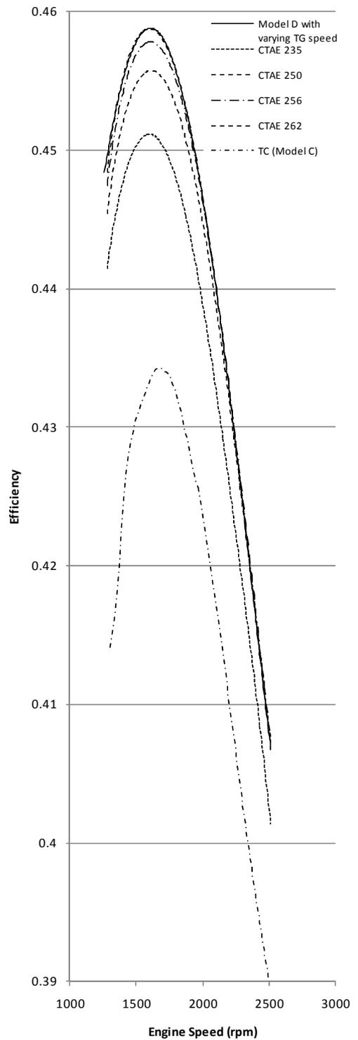
**Figure 14. HOW OVERALL EFFICIENCY IS AFFECTED BY EXHAUST VALVE TIMING**
