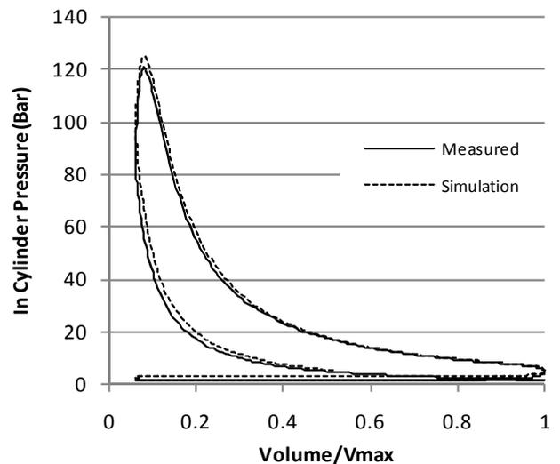
**Figure 3. COMPARISON OF MEASURED AND SIMULATED P-V DIAGRAMS**
