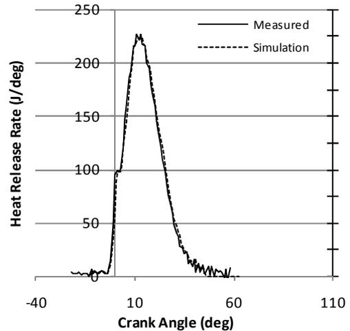
**Figure 2. COMPARISON OF MEASURED AND SIMULATED HEAT RELEASE RATES**
