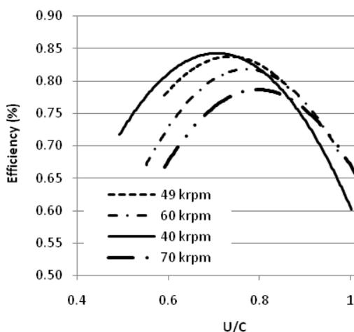
**Figure 12. TURBOGENERATOR TURBINE EFFICIENCY AS FUNCTION OF VELOCITY RATIO**
