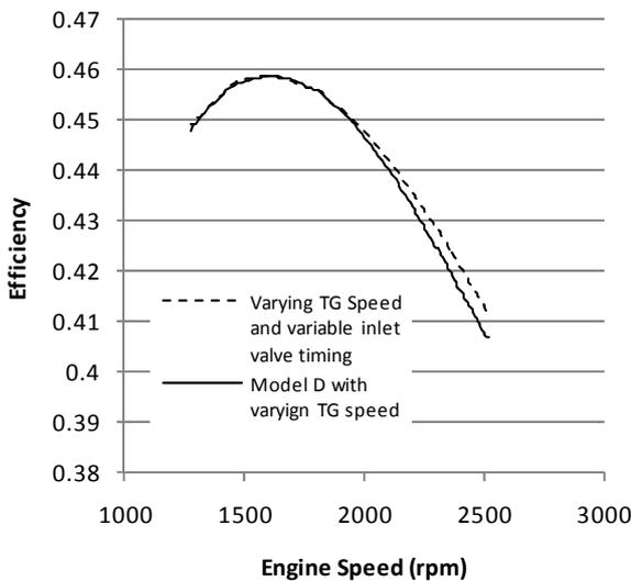
**Figure 15. IMPROVEMENT GAINED BY VARYING TURBOGENERATOR SPEED AS WELL AS VARYING THE INLET VALVE TIMING**
