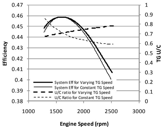
**Figure 11. SYSTEM EFFICIENCY AND TG VELOCITY RATIO**
