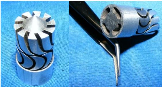
Figure 3 Machined nozzle disk and rotor (1<sup>st</sup> prototype)
