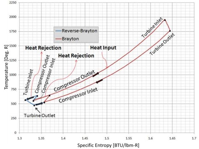
Figure 2. Comparison of the Brayton and Reverse-Brayton cycles.
