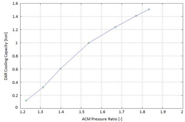
Figure 14. Dry-air-rated ACM cooling capacity.
