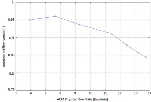
Figure 15. Intercooler effectiveness over operating range of ACM.
