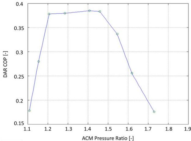
Figure 7. Dry-air-rated COP for the baseline turbocharger.
