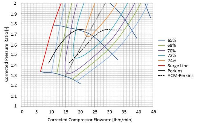
Figure 5. Primary compressor map with operating lines for the Perkins alone and with the ACM operating.
