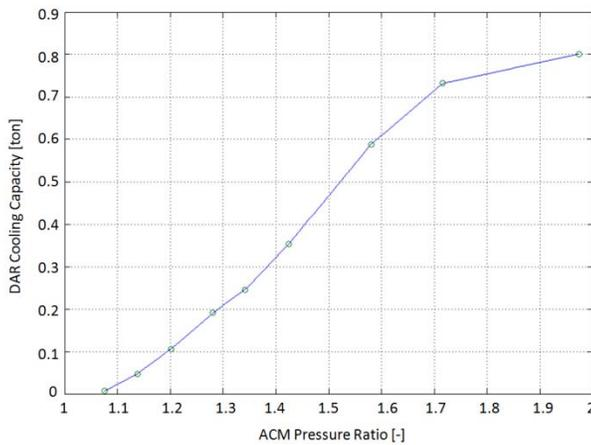
Figure 11. Dry-air-rated ACM cooling capacity.
