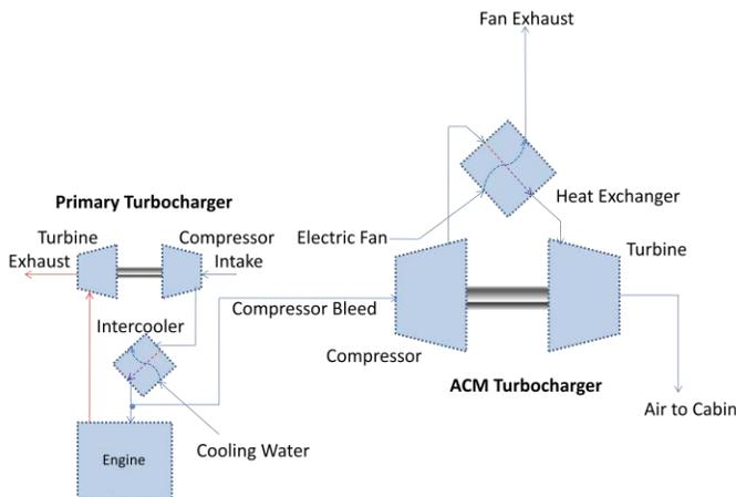
Figure 4. Automotive on-engine schematic of a two-wheel bootstrap ACM configuration.
