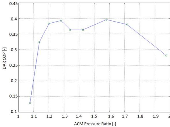
Figure 10. Dry-air-rated COP for the modified ACM turbocharger.
