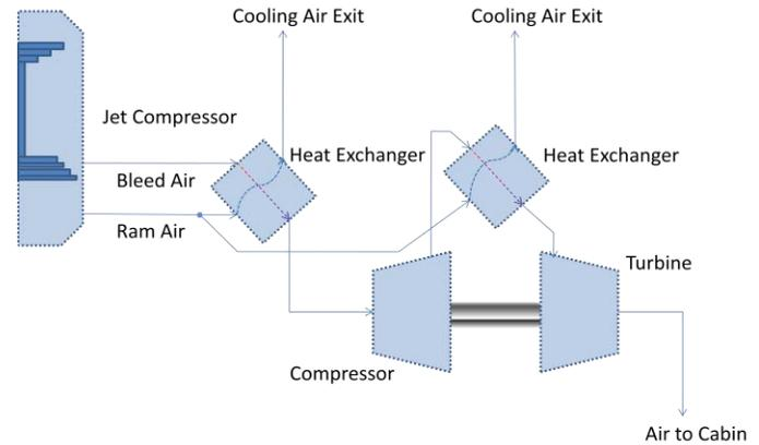
Figure 1. Aircraft schematic of a typical two-wheel bootstrap ACM configuration.
