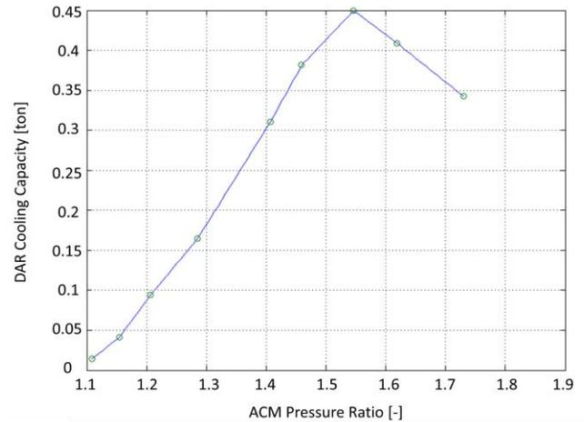
Figure 8. Dry-air-rated ACM cooling capacity for baseline turbocharger.
