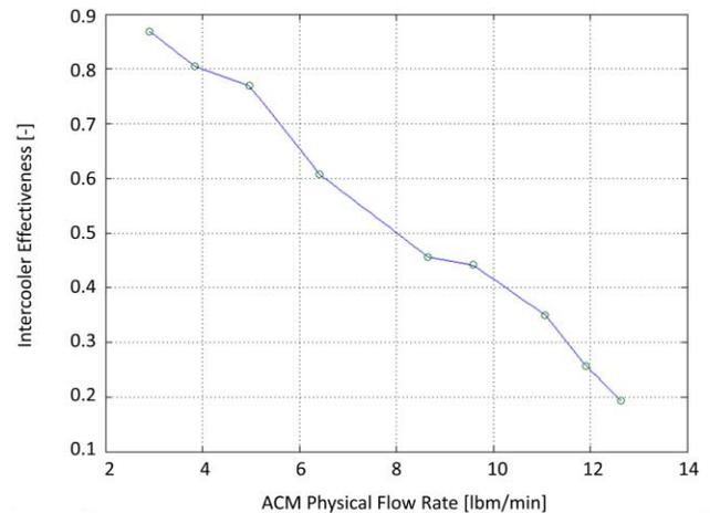
Figure 9. Intercooler effectiveness over operating range of ACM.
