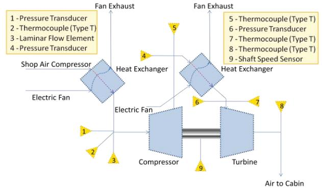
Figure 3. The ACM configured for shop air supply.
