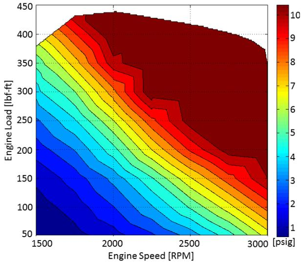
Figure 6. Engine intake manifold pressure baseline on stock turbocharger without the ACM.
