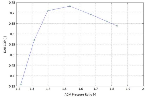
Figure 13. Dry-air-rated COP for the modified ACM turbocharger.
