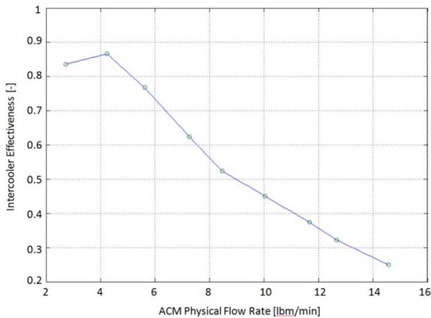
Figure 12. Intercooler effectiveness over operating range of ACM.
