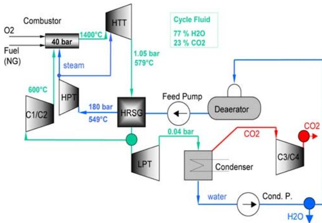
Fig. 1: Principle Process Design for the Graz Cycle Plant [10].
