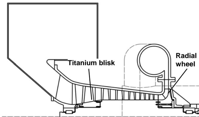
Fig. 5: Graz Cycle Compressor C1 [12]
