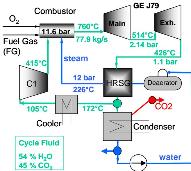
**Fig. 4:** Flow Configuration for a Near-Term Basic Graz Cycle Plant with Fuel Gas Firing (GC-B-J79)
