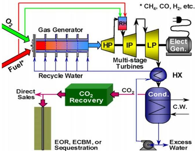
Fig. 2: Principle Flow Scheme of the Oxyfuel CES Cycle [2].
