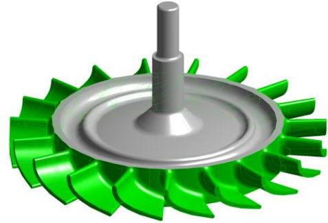
Figure 3. Surfaces where convection condition was applied ( h=627 \text{ W/m}^2\text{K} , 1225°C). Initial rotor temperature was 15°C. The diameter at the blade tips is 58 mm.
