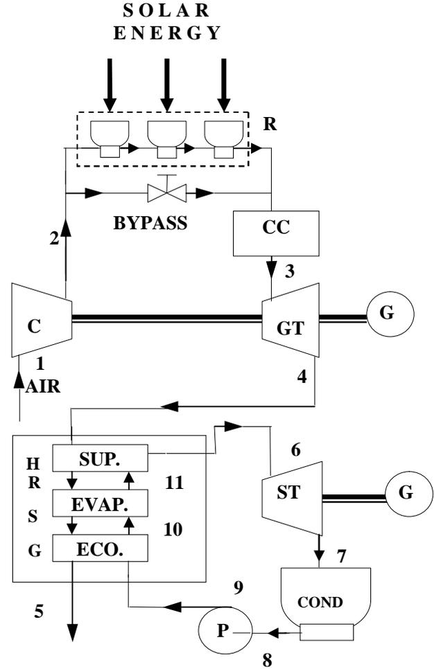
**Fig.1: Schematic of Solar Powered Gas Turbine Plant**
