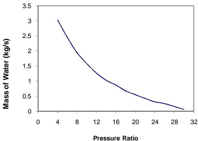
**Fig.6: Variation of mass flow rate of water with pressure ratio**
