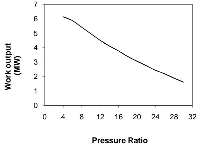
**Fig. 4: Variation of work output with pressure ratio**
