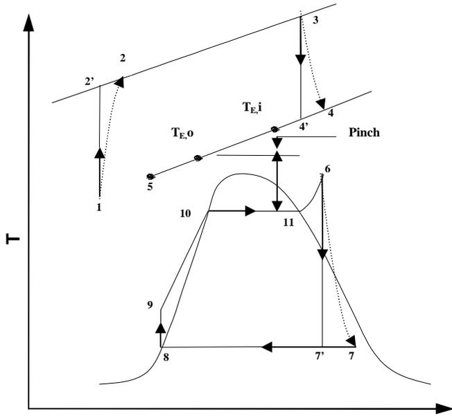
Fig. 3: T-S diagram for the combined cycle
