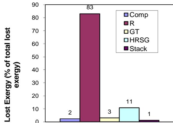
**Fig. 8: Lost exergy of different components at base case pressure ratio 4**
