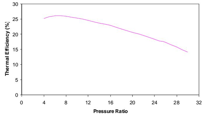
**Fig. 7: Variation of overall thermal efficiency with pressure ratio**
