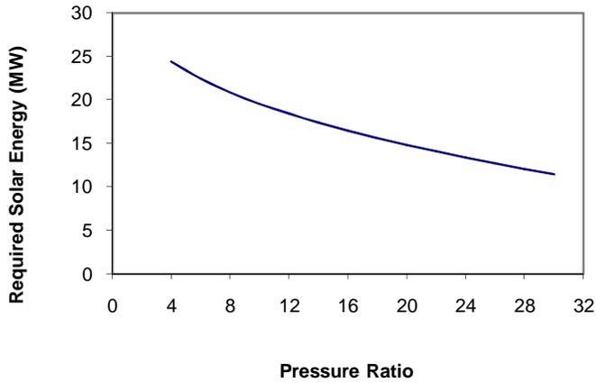
**Fig. 5: Variation of required solar energy with pressure ratio**
