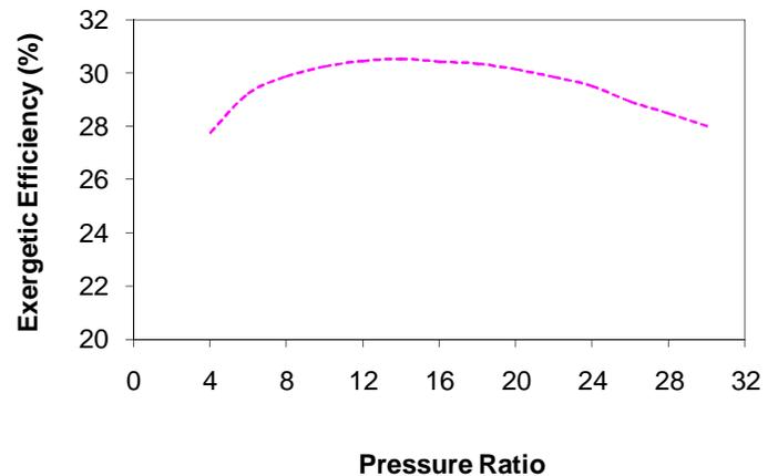
Fig. 11: Variation of overall exergetic efficiency with pressure ratio
