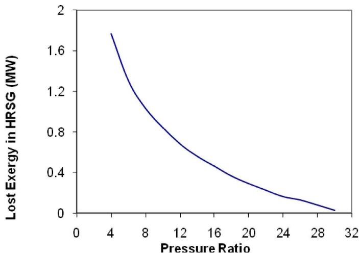
Fig. 10: Variation of lost exergy in HRSG
