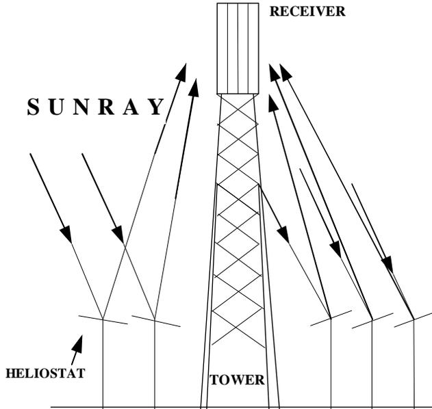
Fig. 2: Schematic of Central Receiver System
