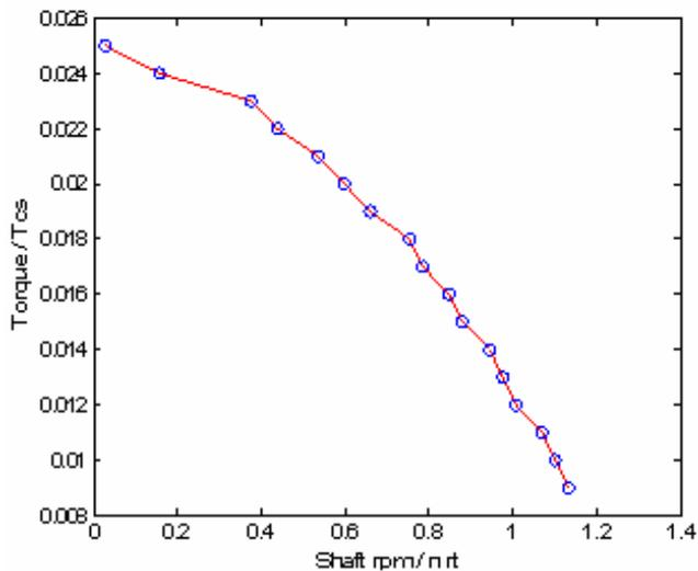
Fig 9:- Variation in Non-dimensional torque transfer with speed through the spur gear side interference fit.
