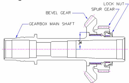
**Fig 2:- Gearbox main shaft, bevel –spur gear arrangement**
