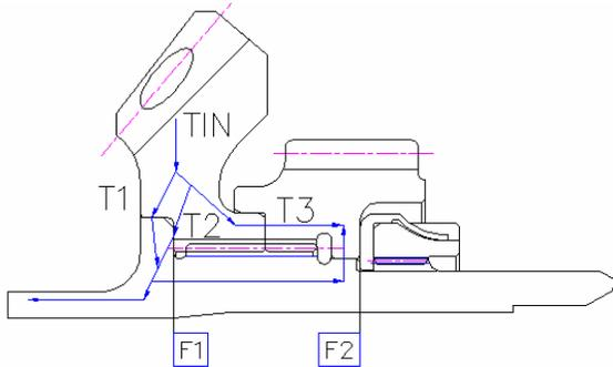
**Fig 4:- Input torque triple split.**
