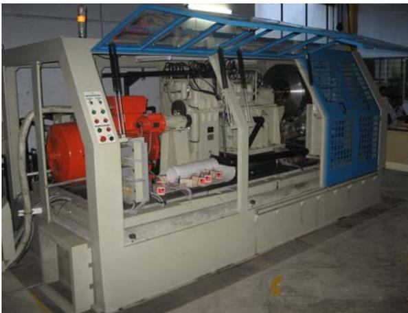
**Fig 11:- Four square back to back test set up**
