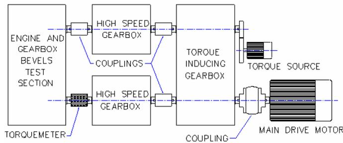
**Fig 10:- Schematic diagram of four square back to back test set up**
