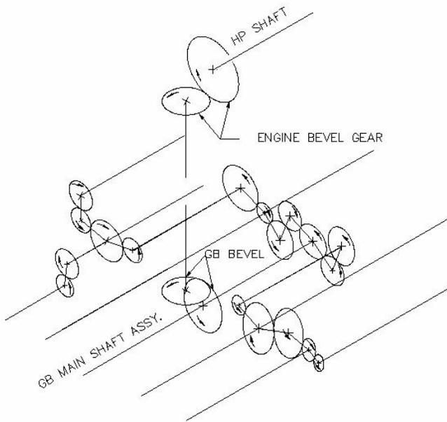
**Fig1:- Engine gearbox gear train with HP shaft**
