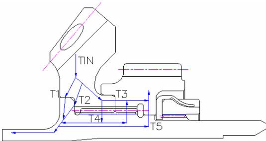
**Fig 5:- Input torque quadruple split.**
