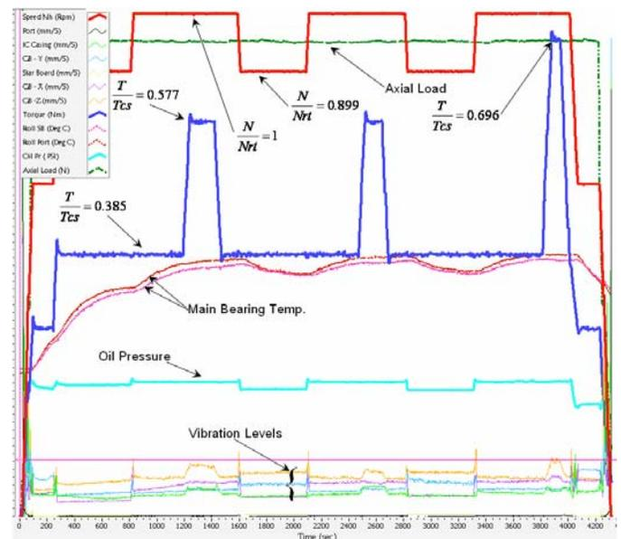
**Fig 13:- Plot for the simulated normal operating condition**
