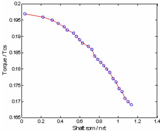
Fig 8:- Variation in Non-dimensional torque transfer with speed through the bevel gear side interference fit.
