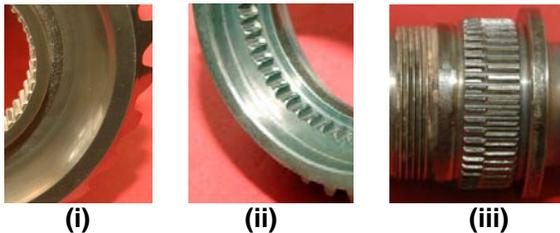
**Fig 3-: (i)-shows the fretting wear on the bevel gear butting face, (ii & iii) - shows the spline wear out**
