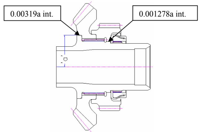
Fig 7:- Interference fit at the collars of the assembly
