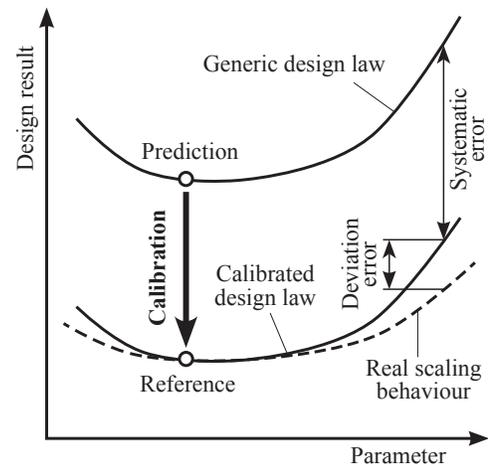
FIGURE 4. Necessity for calibration in preliminary design [4]
