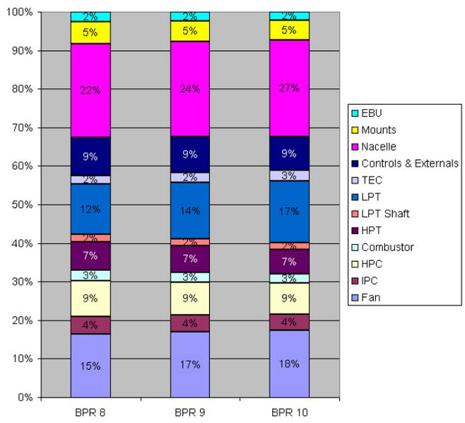
FIGURE 8. Component Mass fractions on Total Engine Mass
