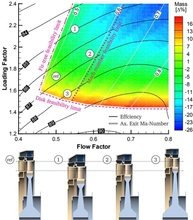
**FIGURE 3.** Aerodynamical Design Space of a Turbomachinery according to [4]
