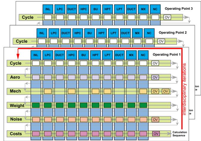
FIGURE 2. Modularity and calculation sequence of MOPEDS according to [14]
