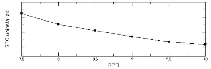
FIGURE 6. Specific Fuel Consumption vs. BPR
