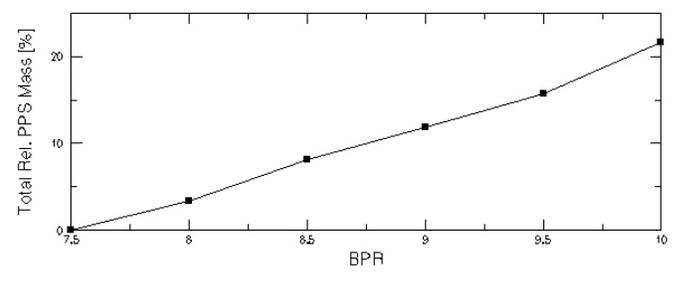
FIGURE 10. Relative Propulsion System Mass vs. BPR
