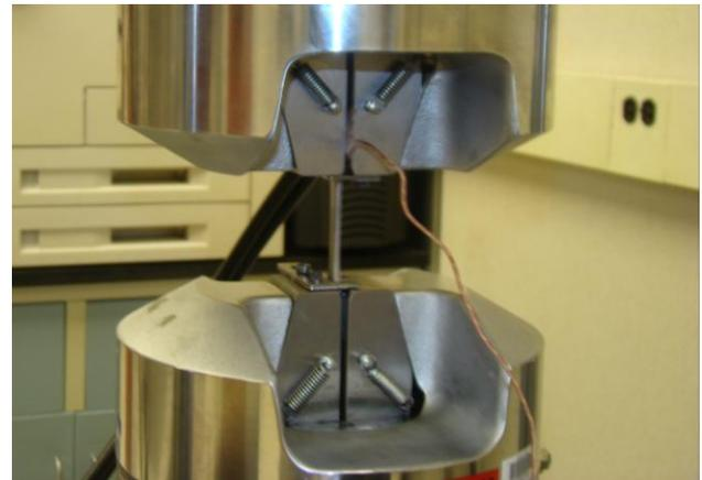
Fig. 7. Test set up of wedge and thermal couple.
