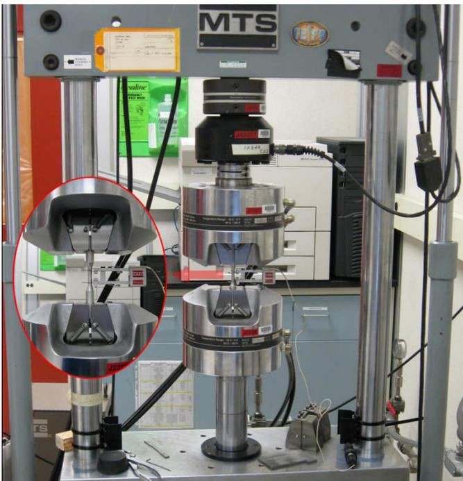
Figure 4. MTS machine with extensometer
