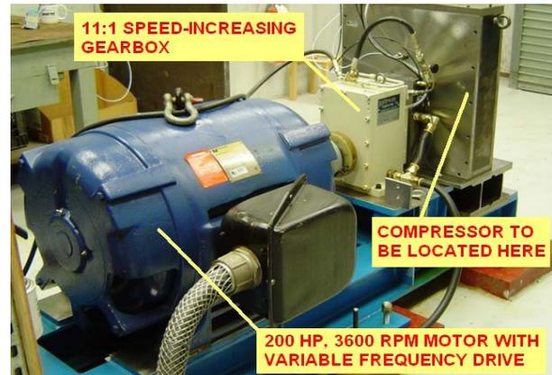
**Figure 7. Experimental test rig with motor and gearbox.**
