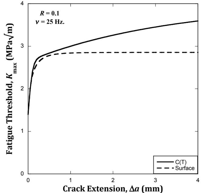
FIGURE 4. CALCULATED  $R$ -CURVE FOR SEMI-ELLIPTICAL SURFACE CRACK PLOTTED WITH MEASURED  $R$ -CURVE FOR A COMPACT TENSION SPECIMEN
