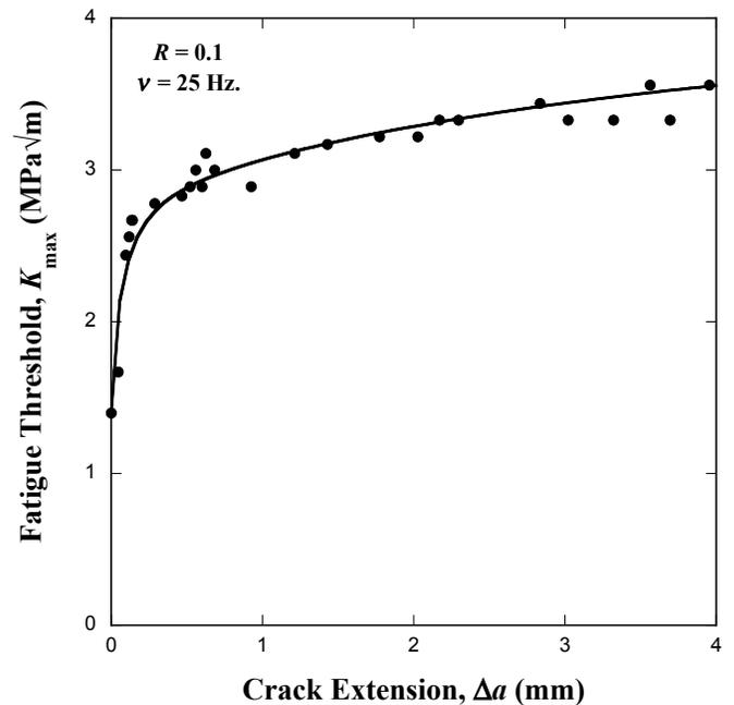
**FIGURE 2. MEASURED FATIGUE THRESHOLD  $R$ -CURVE**
