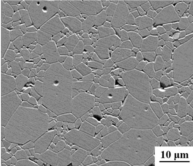
**FIGURE 1. SCANNING ELECTRON MICROGRAPH OF THERMALLY ETCHED SURFACE OF POLYCRYSTALLINE ALUMINA USED IN THIS STUDY, COORSTEK AD995.**
