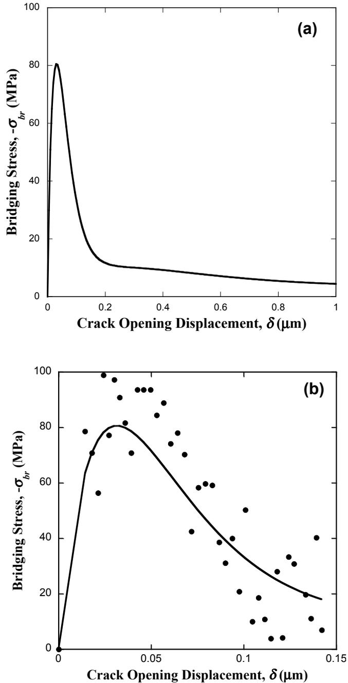
FIGURE 3. (a) CALCULATED BRIDGING STRESS PROFILE (SOLID LINE) FOR AD995 WITH (b) MEASURED BRIDGING STRESSES (SOLID CIRCLES)
