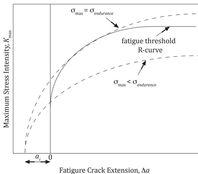
**FIGURE 5. SCHEMATIC FOR DETERMINING THE FATIGUE ENDURANCE STRENGTH FOR A GIVEN INITIAL FLAW SIZE**
