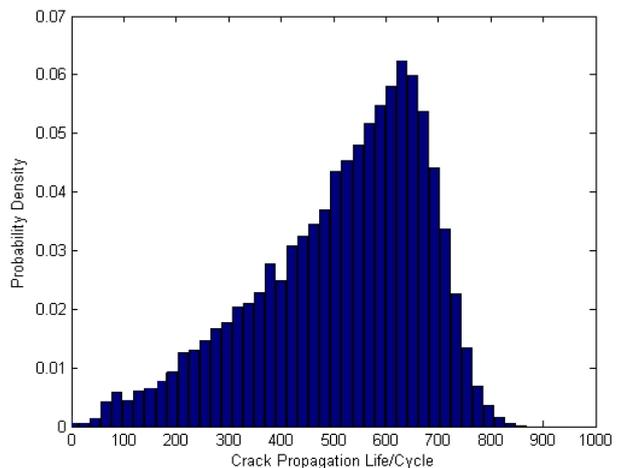
**FIGURE 9** Lifetime histogram by effect of random  $\omega$  and  $a_0$  (crack length 0.39-1.8mm)
