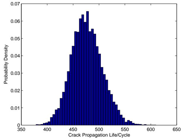
**FIGURE 8** Lifetime histogram by effect of random  $\omega$  (crack length 0.39-1.8mm)
