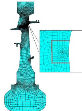
**FIGURE 3** Two-dimensional turbine disk FE model
