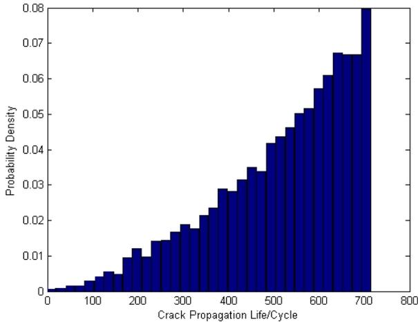
**FIGURE 7** Lifetime Histogram by effect of random  $a_0$  (crack length 0.39-1.8mm)
