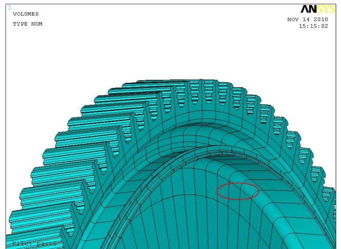
FIGURE 1 Failure Crack Location
