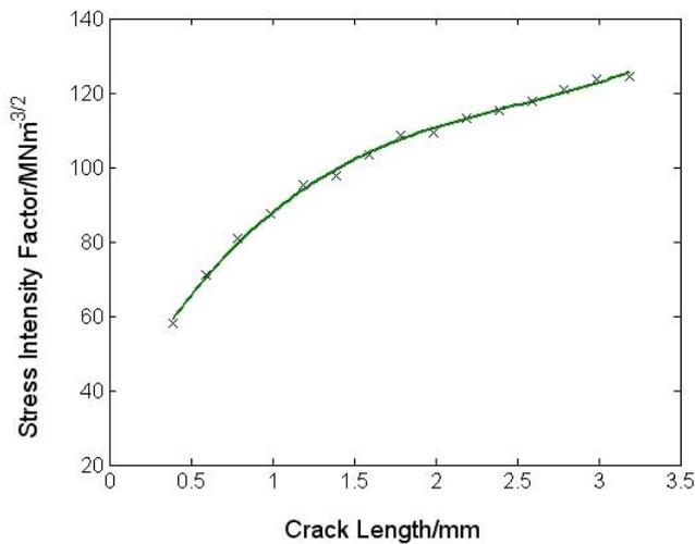
FIGURE 5 Relationship between Crack Length a and Stress Intensity Factor K
