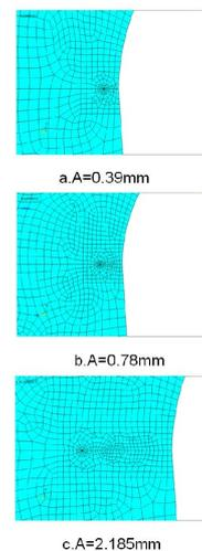
**FIGURE 4** Crack Tip FE Model of Different Length
