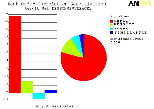
**FIGURE 6** Sensitivity of SIF ( $a=0.79mm$ )
