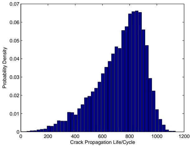
**FIGURE 10** Lifetime histogram by effect of two random parameters (crack length 0.39-3.2mm)
