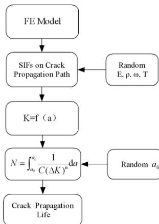
**FIGURE 2** Process of Probabilistic Life Analysis
