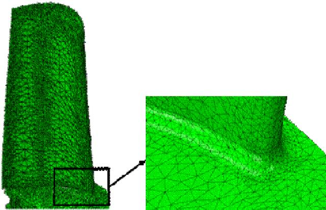
**Figure 1:** Uncooled turbine vane used for the investigation and its LE fillet
