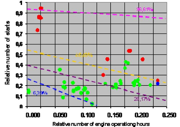
**Figure 5:** Damage diagram vs. probability of damage in at least one vane in a row. Green circles correspond to crack absence, red ones to LCF micro crack presence and blue ones to creep pores (micro crack)
