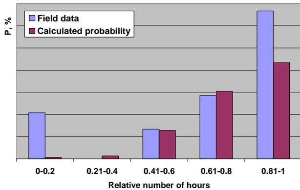
**Figure 7:** Comparison between field statistics and results of probabilistic analysis for vane rows having at least one vane with micro crack depending on the relative number of operating hours.
