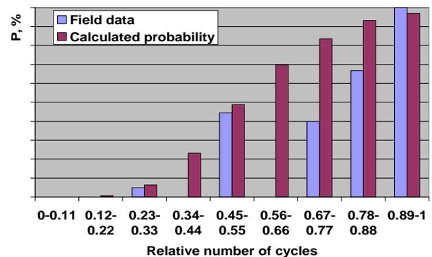
**Figure 6:** Comparison between field statistics and results of probabilistic analysis for vane rows having at least one vane with micro crack depending on the relative number of starts.
