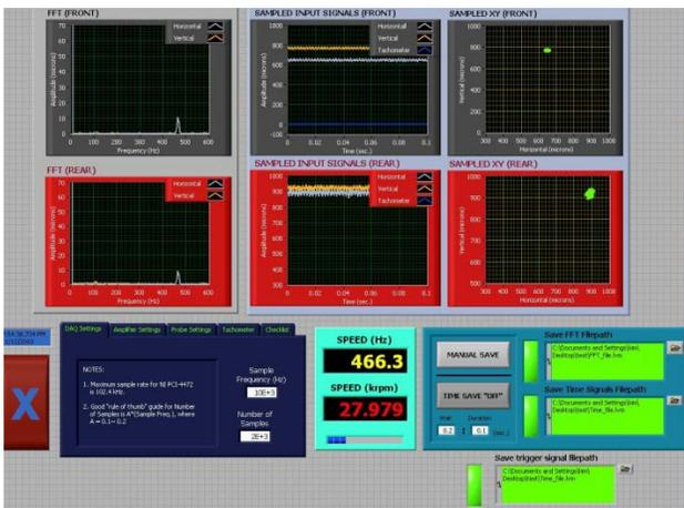
Figure 5 Screen capture of Labview-based in-house rotordynamic software
