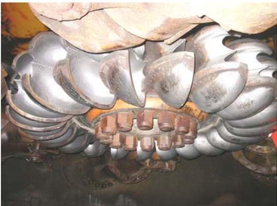
Figure 3. Pelton runner equipped with 21 buckets.
