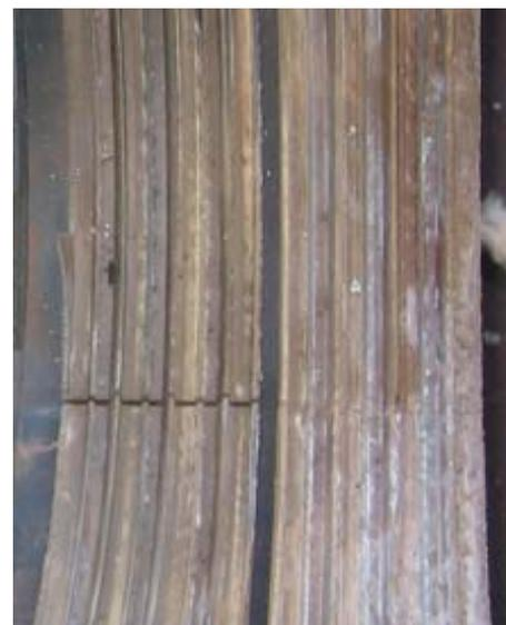
**Figure 19.** Labyrinth seal after overhaul.
