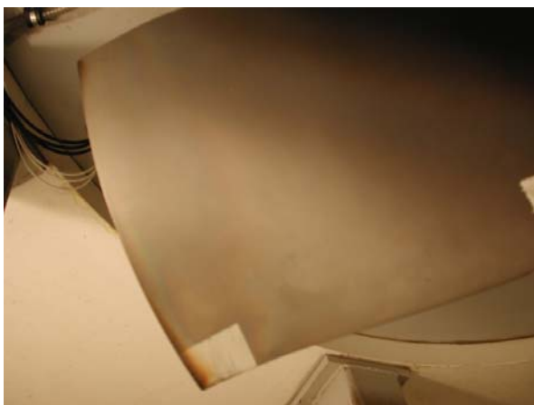
Fig. 11 Close-up of the tip of the blade after several rub experiments.
