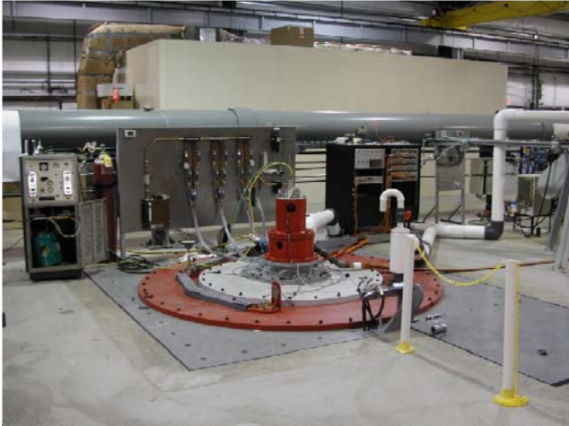
Fig. 1 View of the Large Spin Pit Facility: (a) the containment tank during construction and (b) the facility in operation.
