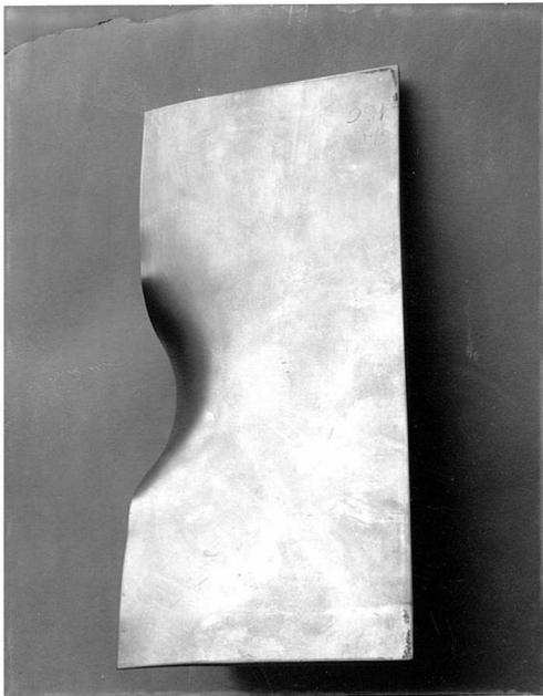
**FIG. 1: A typical plastically deformed bulge in the leading edge of a metal turbfan blade after slicing action during bird-strike**
