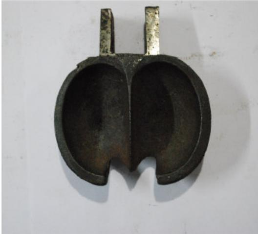
Figure 10 Fabricated Bucket
