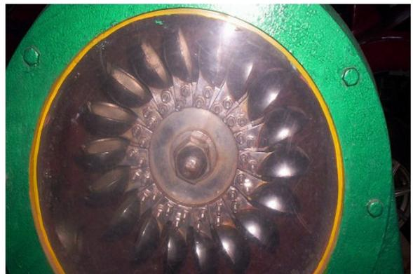
Figure 14 Traditional Pelton Runner Fitted At the Test Rig
