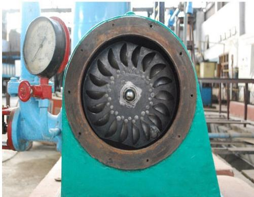
Figure 15 Hooped Pelton runner Fitted At the Test Rig
