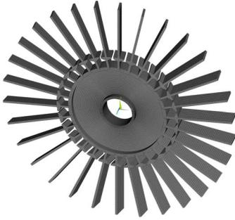
**FIGURE 7.** FINITE ELEMENT MODEL OF A MODEL BLISK WITH 30 BLADES AND 82080 DEGREES OF FREEDOM.
