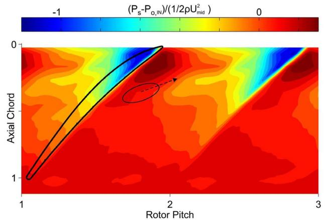
FIGURE 4. Casing static pressure contours near stall.
