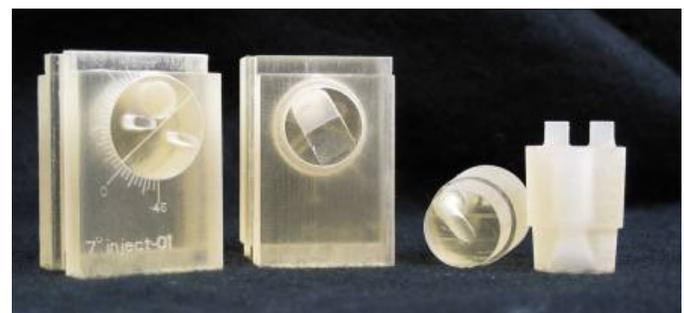
**FIGURE 17.** Pieces for injection nozzle testing driven by an external air supply.
