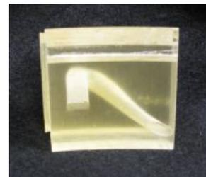
**FIGURE 19.** Inner detail of casing treatment loop segment.
