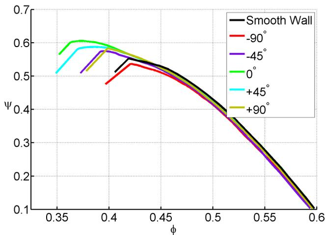
**FIGURE 18.** Pressure rise characteristic for various injection angles. Twelve slot injectors with  $V_i/V_x = 2$ .
