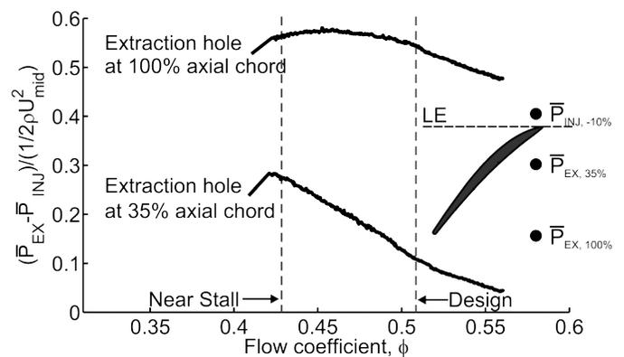
**FIGURE 7. Measured characteristics of driving pressure for injection hole at 10% axial chord upstream of leading edge and for extraction holes at 100% chord and 35% chord.**
