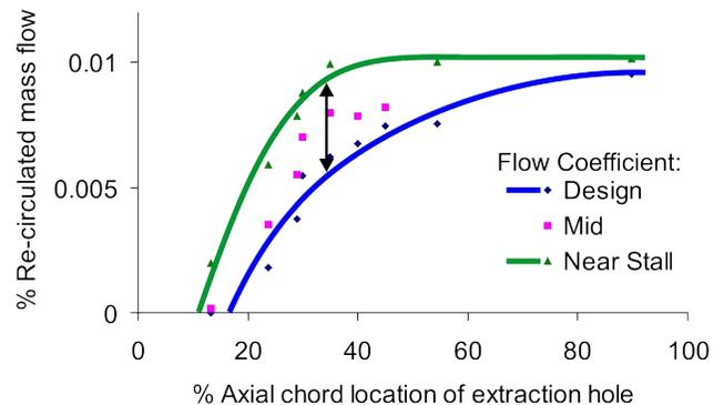
**FIGURE 11. Extraction hole optimization: axial chord location.**
