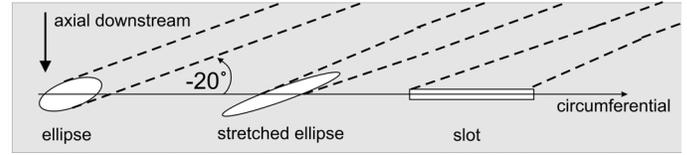
FIGURE 13. Extraction hole geometries viewed on casing surface.
