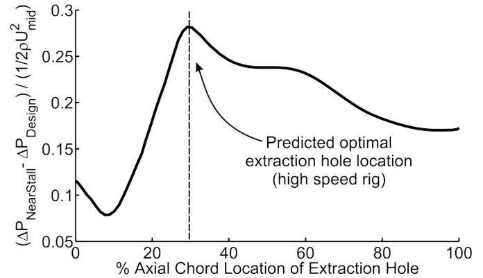
**FIGURE 22. “Sweet spot” for extraction hole location in a high speed compressor predicted from re-circulation loop driving pressure ( $\Delta P = \bar{P}_{EX} - \bar{P}_{INJ}$ ) at near stall and design conditions, as explained for Fig. 6. Driving pressure is based on CFD casing pressure calculations.**
