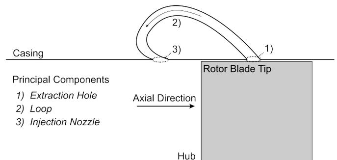
FIGURE 1. New extraction/re-injection casing treatment design.
