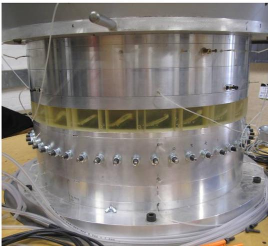
**FIGURE 15.** Photo of Mini-Deverson compressor with casing treatment (transparent ring) installed.
