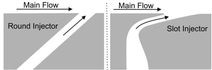
**FIGURE 16.** Injection Nozzle Designs.
