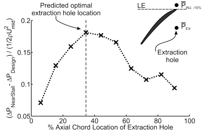
**FIGURE 6. “Sweet spot” for extraction hole location predicted from re-circulation loop driving pressure ( $\Delta P = \bar{P}_{EX} - \bar{P}_{INJ}$ ) at near stall and design conditions. Driving pressure is based on over-tip static pressure measurements (Figs. 2 and 4).**
