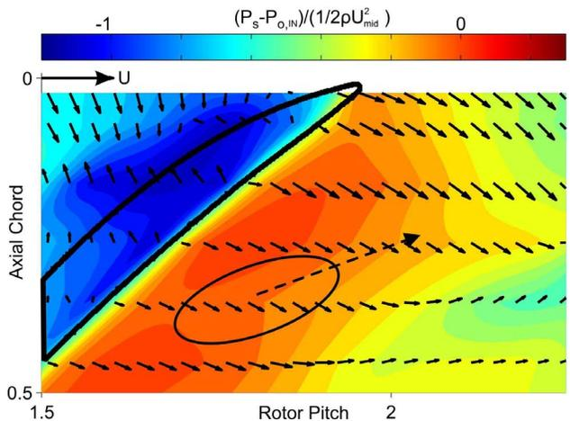
FIGURE 3. Casing static pressure contours at design with absolute velocity vectors at 50% tip clearance height.
