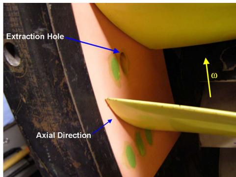
**FIGURE 9. Compressor casing with composite block and extraction hole locations viewed from upstream of the rotor.**
