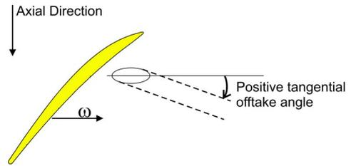
**FIGURE 10. Tangential offtake angle imposed on the casing surface viewed from the hub.**
