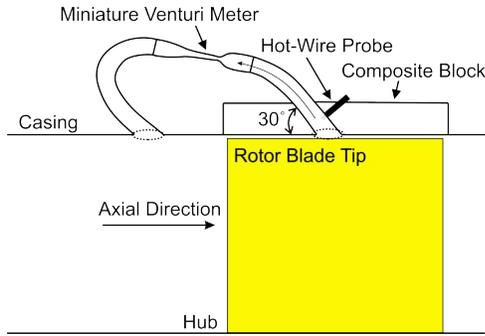
**FIGURE 8. Instrumented extraction/re-injection loop.**
