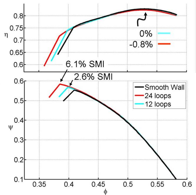
**FIGURE 21.** Efficiency and pressure rise characteristics for extraction/re-injection loops with rotor blades stagger increased 2°.
