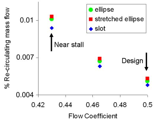
FIGURE 14. Extraction hole geometry optimization.
