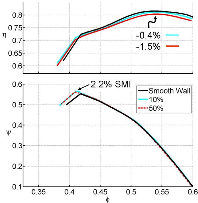
**FIGURE 20.** Efficiency and pressure rise characteristics for 12 extraction/re-injection casing treatment loops. The injectors are placed at 10% and 50% axial chord length upstream of the rotor leading edges.
