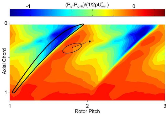
FIGURE 2. Casing static pressure contours at design conditions.
