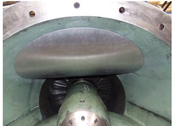
Fig. 23: Bump to simulate inlet distortion
