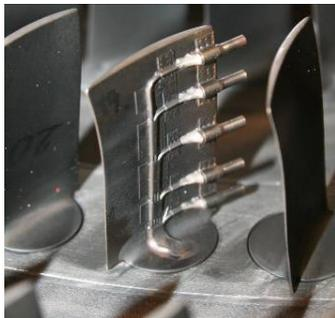
Fig. 17: Variable Stator 3 leading edge total pressure probes
