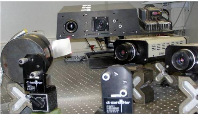
Fig. 6: Laboratory test set-up for natural frequency and mode shape determination
