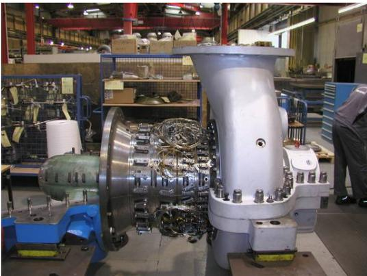
Fig. 1: MAN test rig compressor
