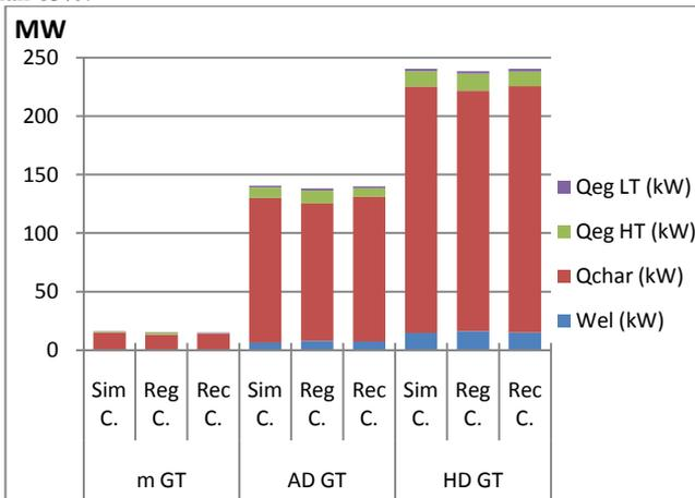
**FIGURE 8. (A) IPRP CHP performance on wheat straw residues from bioethanol production**
