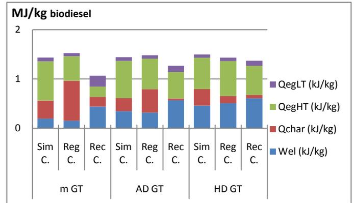
Figure 13. (B) IPRP CHP performance on glycerin from soybean oil biodiesel normalized to 1 kg of biodiesel
