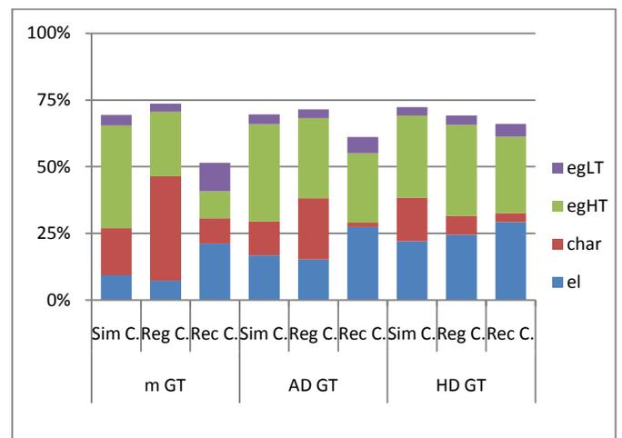
Figure 14. (C) IPRP CHP efficiency on glycerin from soybean oil biodiesel
