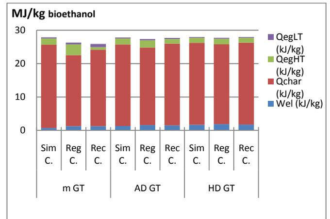
**Figure 9. (B) IPRP CHP performance on wheat straw residues from bioethanol normalised to 1 kg of bioethanol**
