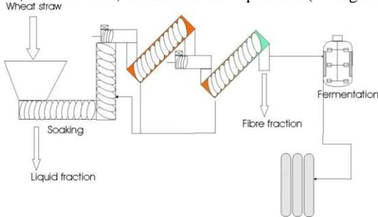
Figure 3. Bioethanol plant layout
