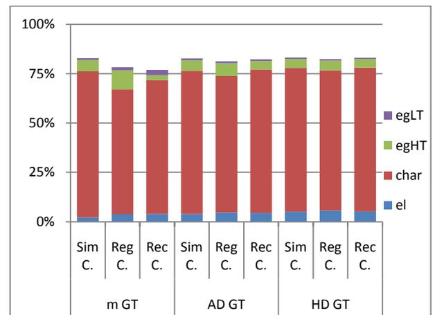
**Figure 10. (C) IPRP CHP efficiency on wheat straw residues from bioethanol**
