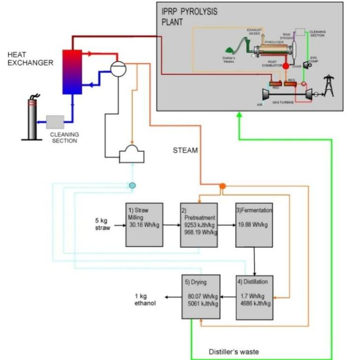
Figure 4. Bioethanol plant mass and energy balance
