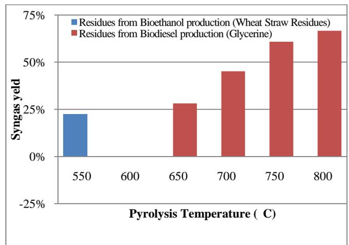
**Figure 7. Syngas production from bioethanol production residues (Wheat straw residues) and from biodiesel production residues (Glycerine) for different  $T_p$**
