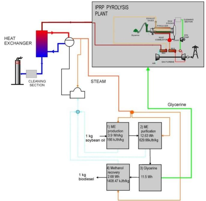
Figure 6. Biodiesel plant mass and energy balances
