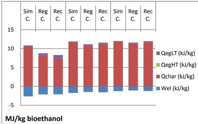
Figure 11. (D) Overall IPRP + Wheat Straw Bioethanol energy output normalized to 1 kg of bioethanol
