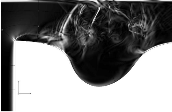
Figure 19 Density gradient contours in a supersonic tip recess
