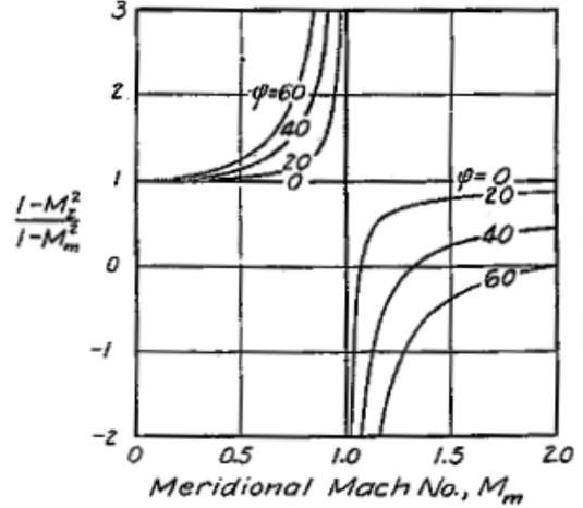
**Figure 4: Streamline curvature gradient singularity shown at  $M_m = 1$  (plot reproduced from Smith [4])**
