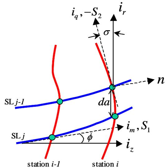
Figure 2: Streamlines and quasi-orthogonals ( $S_2$ ) representation for the throughflow method
