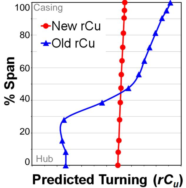
**Figure 7: Plot showing the radial distribution of turning ( $rC_u$ ) for throat station under localized streamtube choking. Red: after correction; Blue: before correction.**
