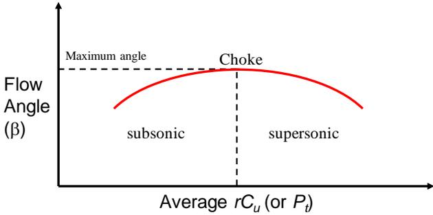
**Figure 3: Variation of bladerow exit flow angle ( $\beta$ ) with average turning ( $rC_u$ ) or total pressure ( $P_t$ )**
