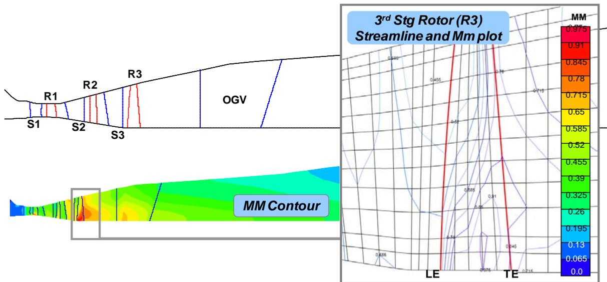
**Figure 9: Predicted meridional Mach number shown for a 3-stage transonic turbine test case. Solution obtained using the numerical improvements presented in this paper.**
