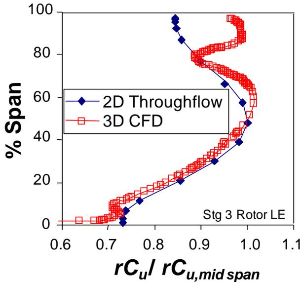
**Figure 10: 3D CFD and 2D throughflow comparison for a transonic 3-stage turbine test case**
