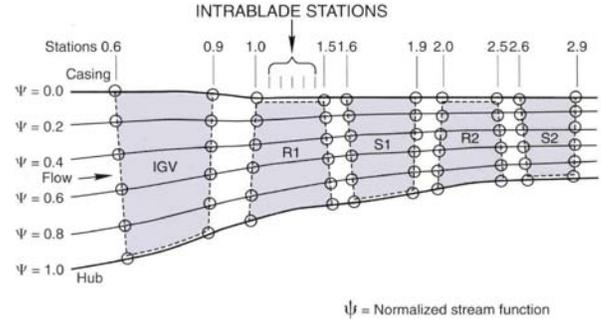
Figure 1: Schematic representation of a throughflow computational grid
