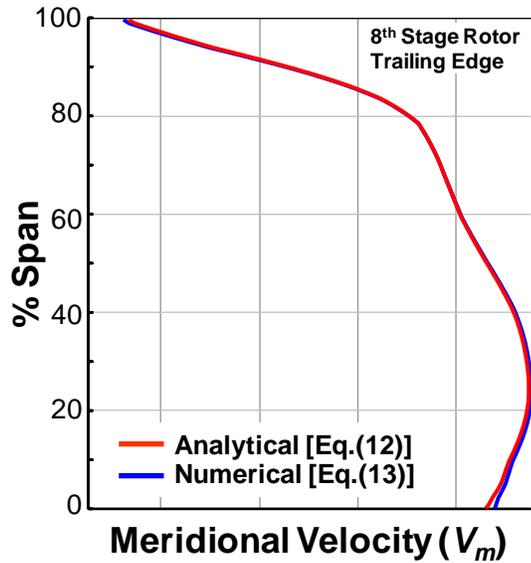
**Figure 8: Meridional velocity distribution at TE of 8<sup>th</sup> stage rotor of the subsonic compressor test case. Results showing solver consistency for a subsonic test case.**
