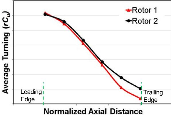
**Figure 6: Sample meanline bladerow turning distribution for two rotors**
