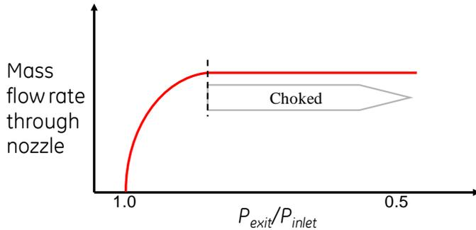
**Figure 5: Variation of mass flow with exit pressure. Plot also shows choked flow condition**
